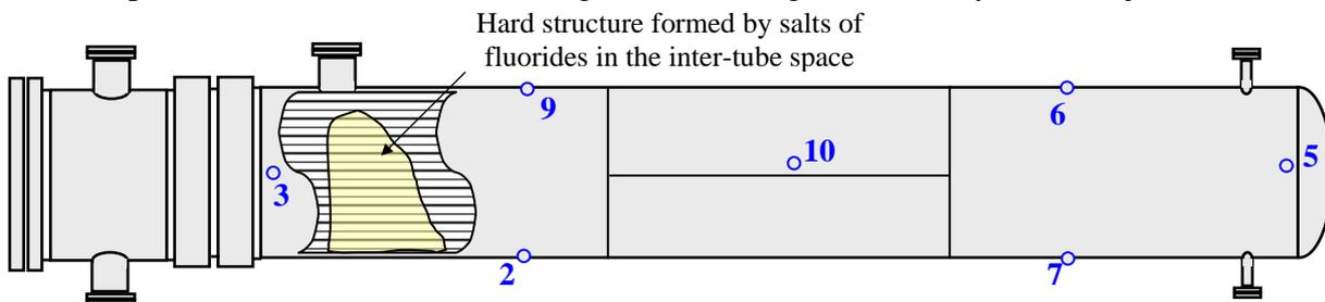
Picture 4. Scheme of heat exchanger contented unexpected object of AE activity.
