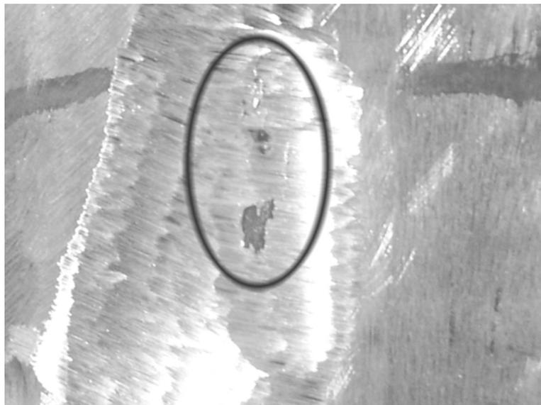
Picture 6. This is the picture of metal defect at the weld of the manhole of the reactor.
