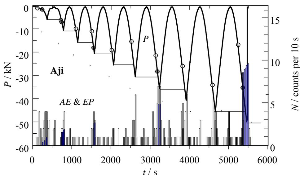
Fig. 7. History of the repeated loading test and the result of AE and EP simultaneous measurement conducted on Aji Granite sample.
