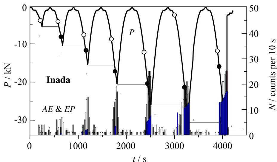
Fig. 6. History of the repeated loading test and the result of AE and EP simultaneous measurement conducted on Inada Granite sample.
