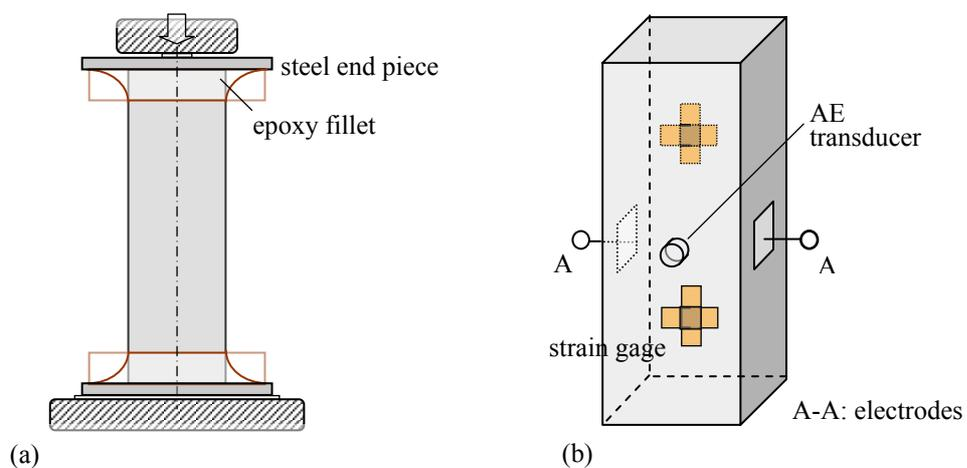
Fig. 5. Sample assembly: (a) setup for uniaxial loading and (b) arrangement of AE transducer, electrodes for EME detection, and strain gages.
