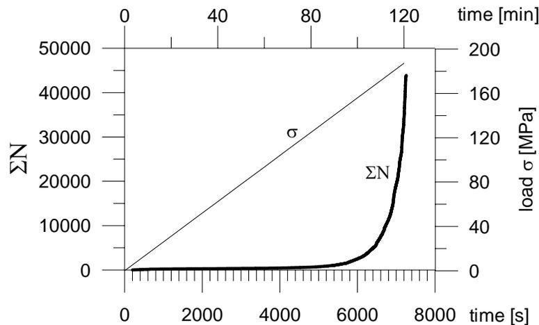
**Fig.1** Loading test, migmatite rock sample. Increase in cumulative number of events  $\Sigma N$  (thick line) with time (load  $\sigma$ ) – thin line.
