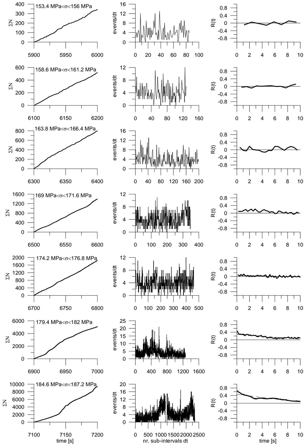
**Fig. 2.** Autocorrelation analysis of UE from loaded rock sample in Fig. 1. First column – cumulative number of events in 100 s intervals. Second column – transformed series of UE events; the length dt of sub-intervals corresponds to average value of 3 events. Third column – autocorrelation coefficients.
