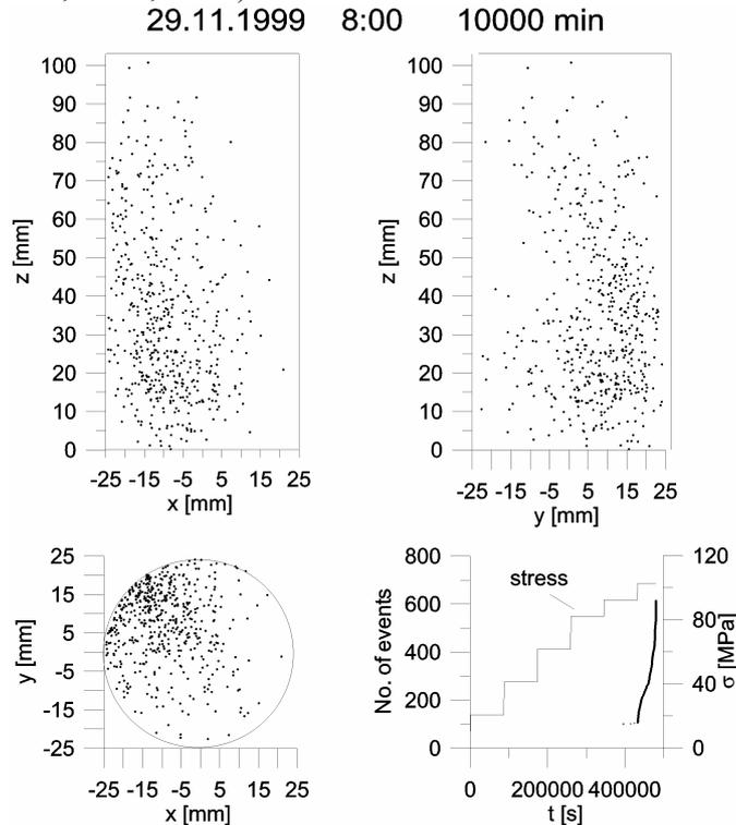
Fig. 4. Graphs of ultrasound emission foci in granite loaded for a period of 10000 minutes, and cumulative graph of the number of events as a function of time and loading.
