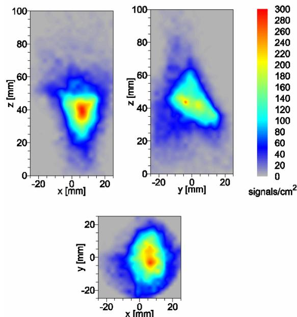
Fig. 6. Distribution of foci of occurrence of the ultrasound emission (events/cm<sup>2</sup>), migmatite 7.
