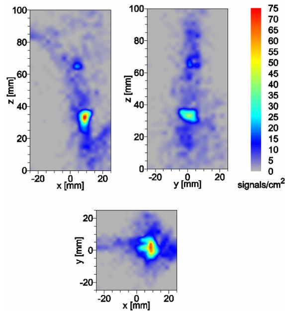
Fig. 5. Distribution of foci of occurrence of the ultrasound emission (events/cm<sup>2</sup>), migmatite 6.
