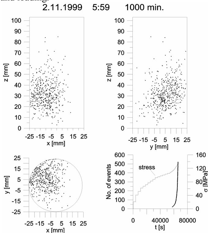
Fig. 3. Graphs of ultrasound emission foci in granite loaded for a period of 1000 minutes, and cumulative graph of the number of events as a function of time and loading.
