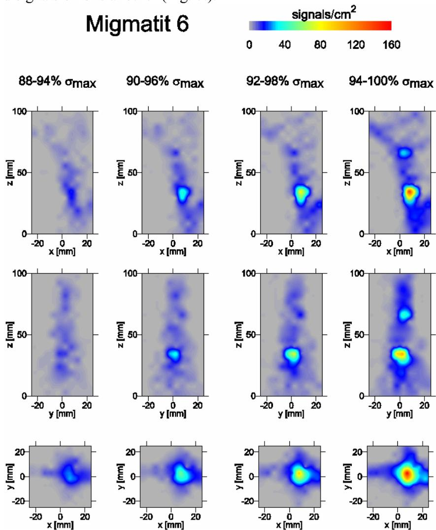
Fig. 7. Distribution of foci of occurrence of the ultrasound emission (events/cm<sup>2</sup>), migmatit 6, evolution of foci in various loading intervals.
