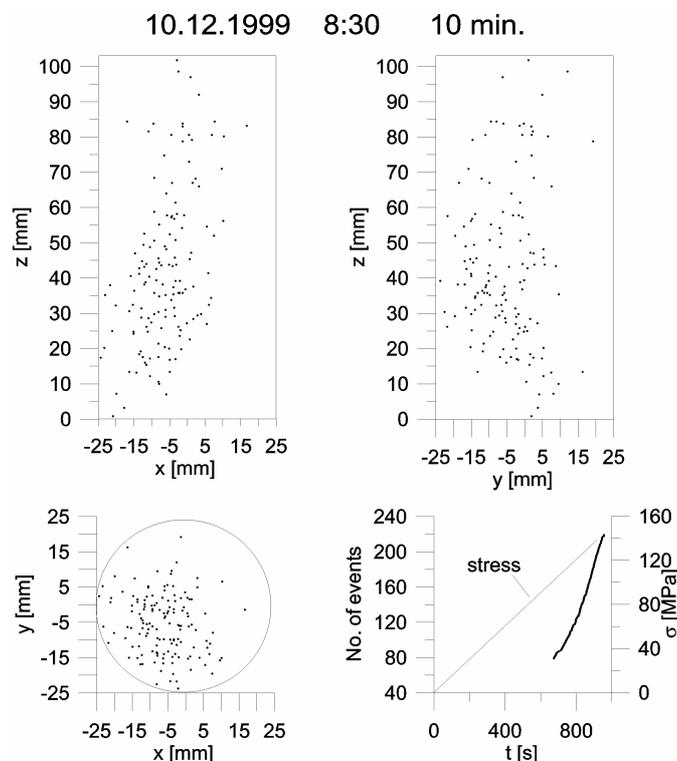
Fig. 1. Graphs of ultrasound emission foci in granite loaded for a period of 10 minutes, and cumulative graph of the number of events as a function of time and loading.
