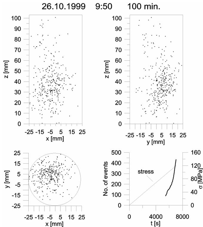
Fig. 2. Graphs of ultrasound emission foci in granite loaded for a period of 100 minutes, and cumulative graph of the number of events as a function of time and loading.
