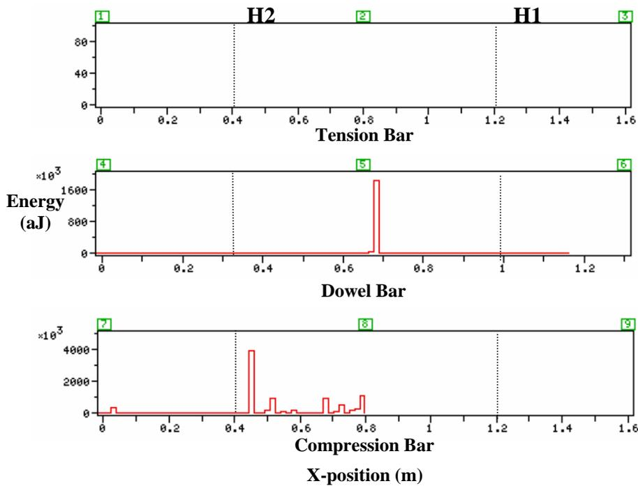
Figure 6: Location of signals detected from sensors attached to steel reinforcement during 250-353kN load stage
