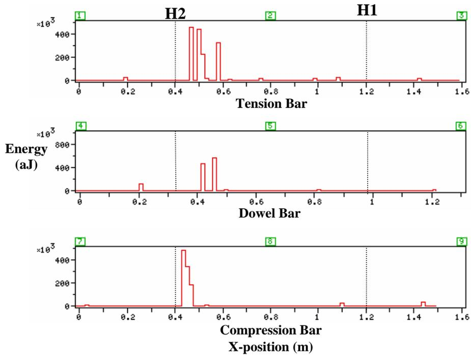
Figure 5: Location of signals detected from sensors attached to steel reinforcement during 10-20kN load stage
