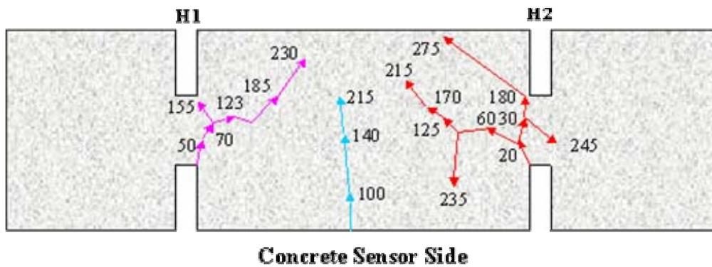
**Figure 3:** Location and direction of cracks with respective loads
