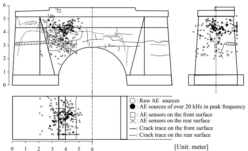
Fig. 3 Arrangement of AE sensors together with 3D AE sources.
