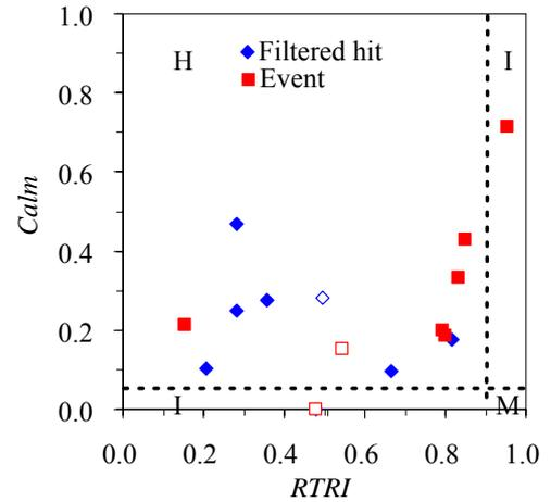
Fig. 10 Calm ratio and RTRI in RC-pier, where 'Event' stands a located source.
