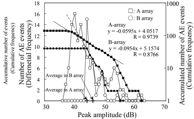
Fig. 12 Amplitude distribution in RC-pier.
