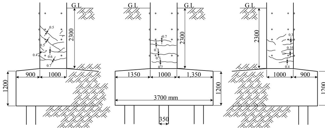
Fig. 4 Crack traces observed in RC-pier, showing north, east and south side from left to right.
