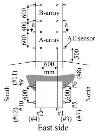
Fig. 5 AE sensor array.
