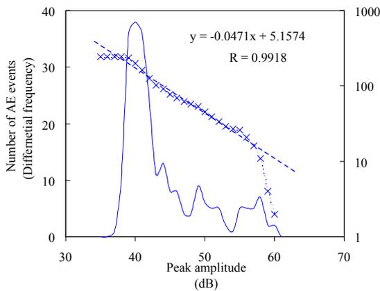
Fig. 11 Amplitude distributions in C-pier.
