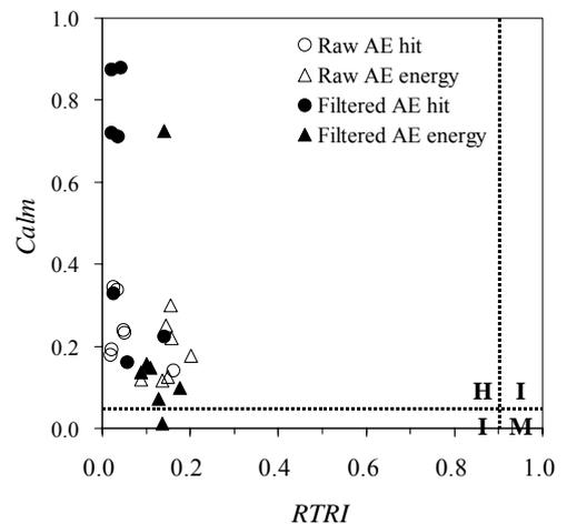
Fig. 9 Calm ratio and RTRI in C-pier, showing H: heavily damage, I: intermediately damage and M: moderately damage.
