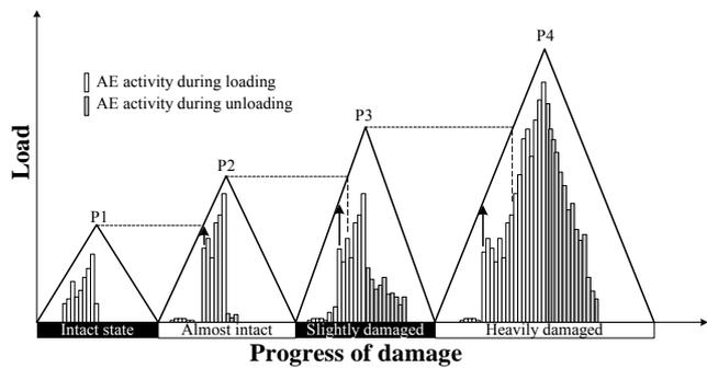
Fig. 1 Representation of AE activity with damage progress.
