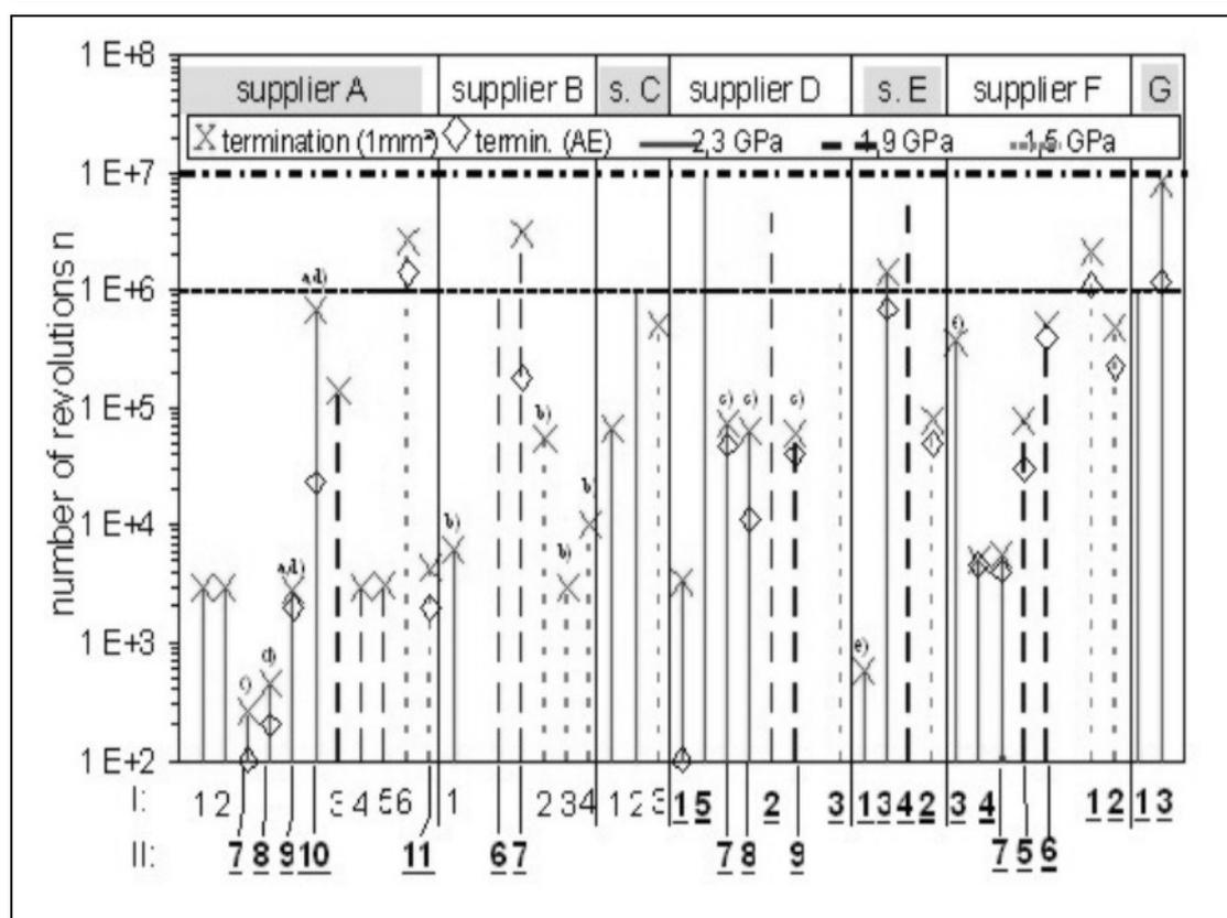
Figure 4: Results of the wear tests of the DLC coating under lubricated slip-rolling friction. Test samples monitored by AE are marked bold and are underlined. In all tests which were terminated (1 mm<sup>2</sup>-criterion), high AE activities (AE criterion) were observed, too.
