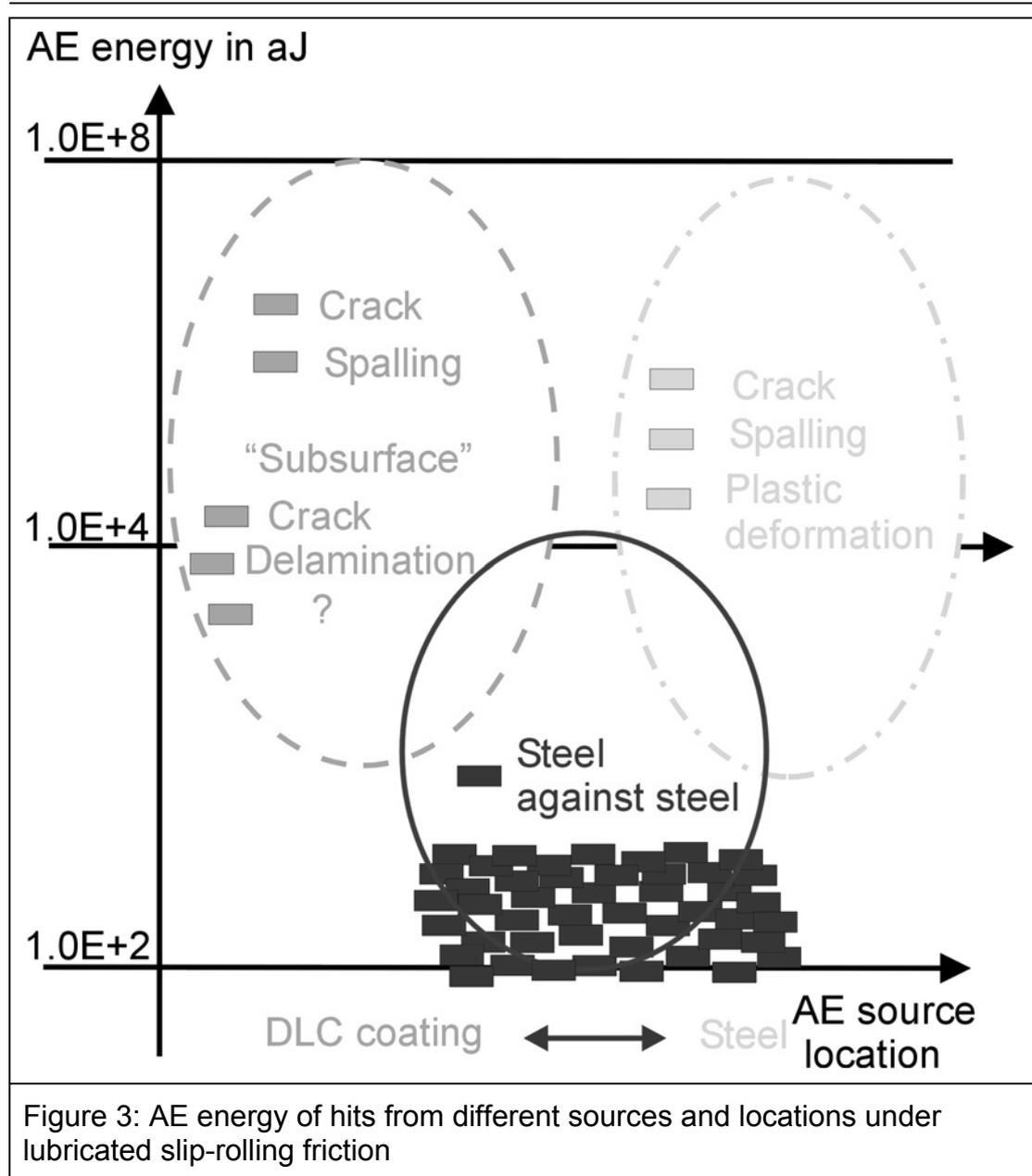
Figure 3: AE energy of hits from different sources and locations under lubricated slip-rolling friction
