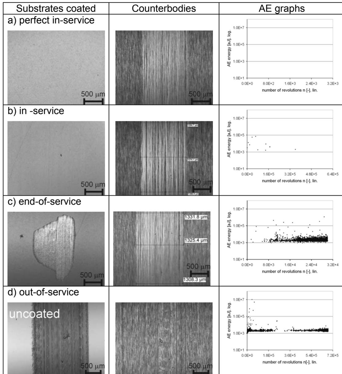
Figure 2: AE indicated the different stages of the wear life of DLC coatings in steel contact under slip-rolling friction. The undesirable contact between steel against steel was indicated immediately by a high AE activity (base noise).
