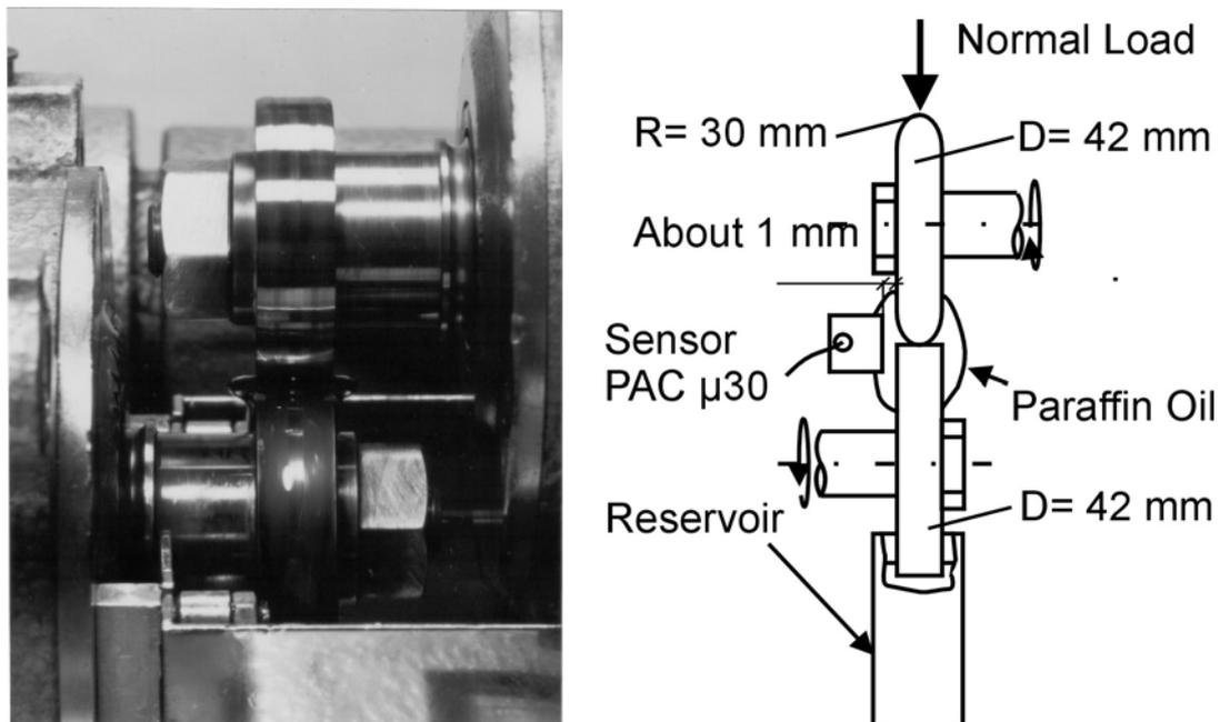
Figure 1: Picture of a test sample in the Amsler type twin-disc wear tester and sketch of the acoustic coupling of the AE sensor under lubricated slip-rolling friction.
