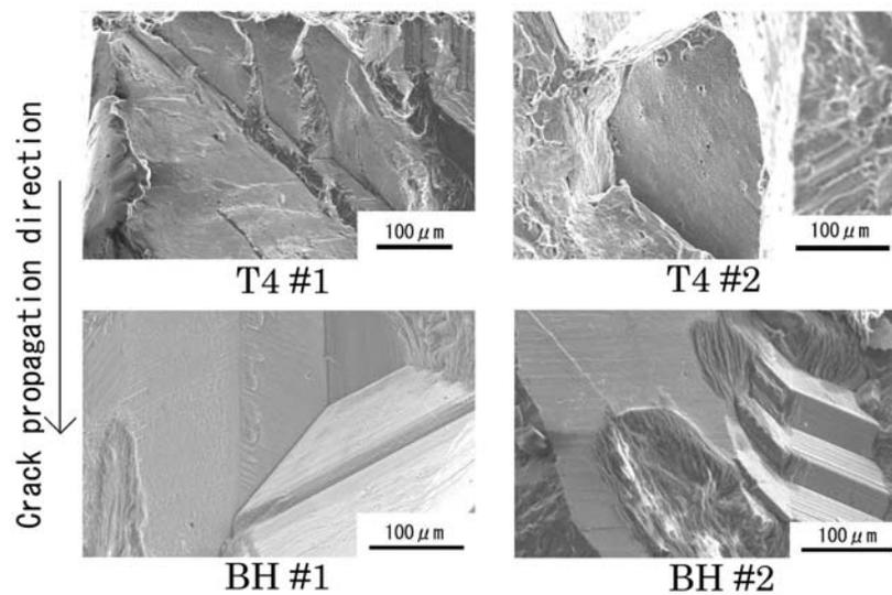
**Fig. 5 Fracture surfaces near the notch point.**
