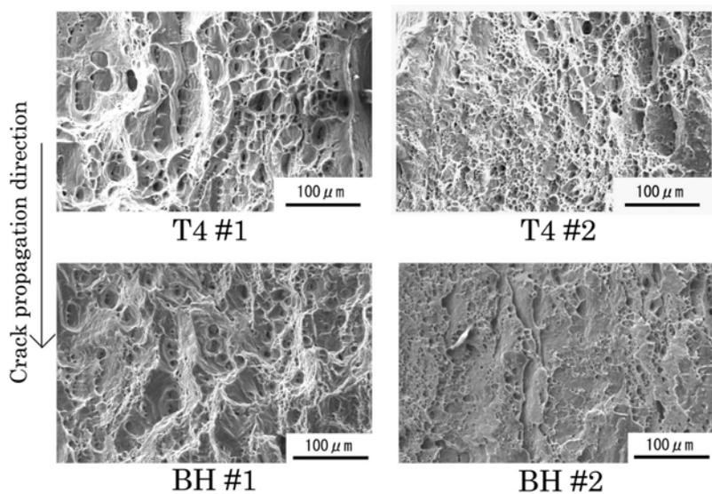
**Fig.7 Fracture surfaces near the final fracture point.**
