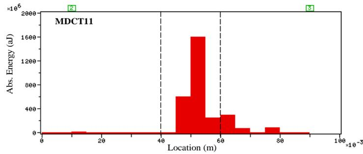
Figure 12 : Example Linear Location on a CT specimen
