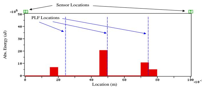
Figure 4 : Location of PLF's between Two Sensors
