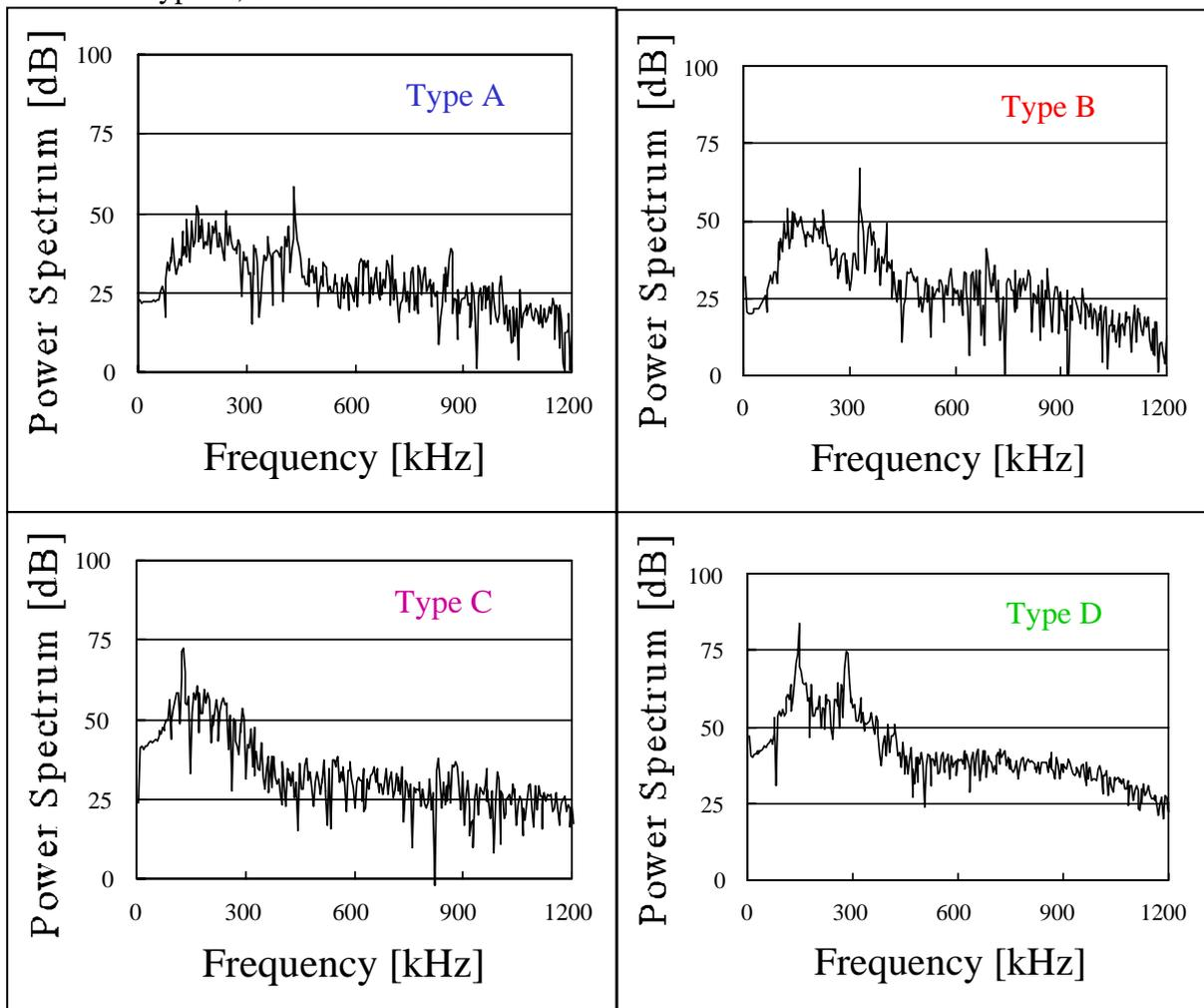
Fig. 7 Frequency spectra of detected AE waveforms at the pressure of 0.30MPa from slit shapes of type A, B, C and D, respectively
