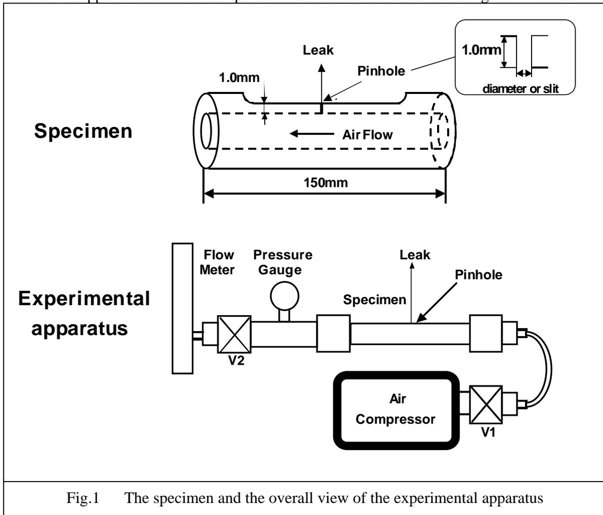
Fig.1 The specimen and the overall view of the experimental apparatus
