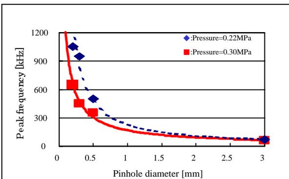
Fig. 5 Relation between the pinhole diameter and the peak frequency of the screech tone
