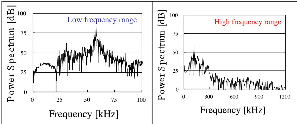
Fig. 3 Frequency spectra of detected AE waveforms at the pressure of 0.30MPa in the frequency range of 20kHz to 100kHz and 100kHz to 1200kHz from the pinhole diameter of 3.0mm
