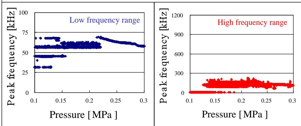
Fig. 4 Relation between the pressure and peak frequency in the frequency range of 20kHz to 100kHz and 100kHz to 1200kHz for the pinhole diameter of 3.0mm
