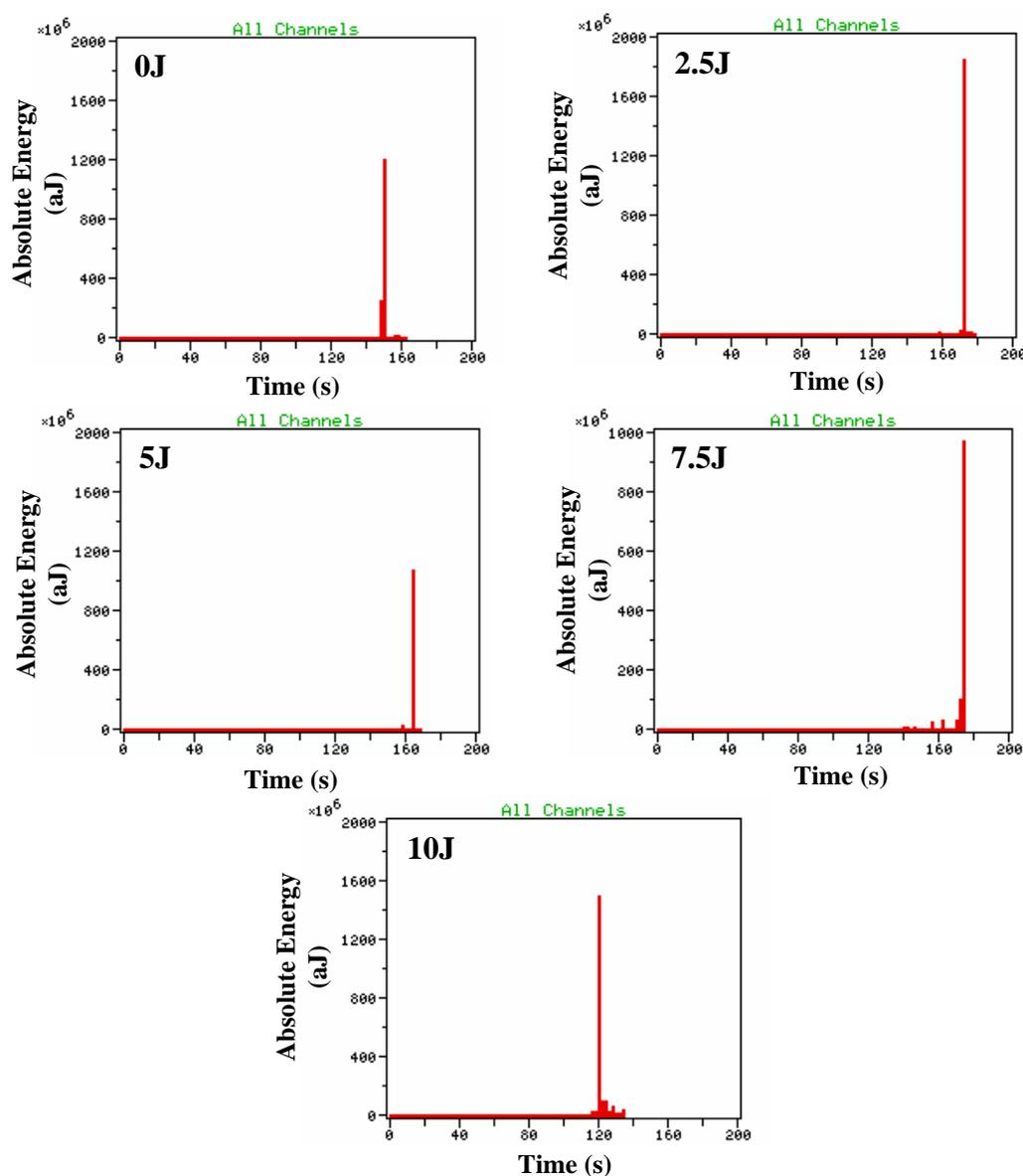
**Figure 3:** Activity of composite plates during loading
