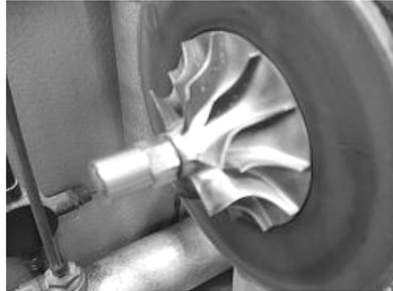
Figure 4: Gas generator compressor impeller.
