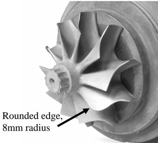
Figure 3: Free-power turbine impeller, damaged blade shown.
