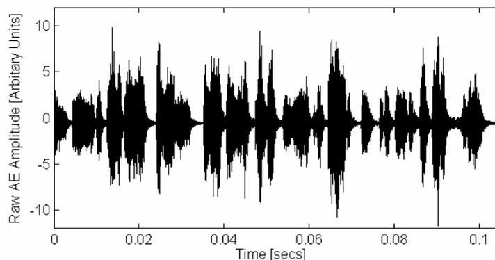
Figure 10: Insufficient fuel supply / unstable running
