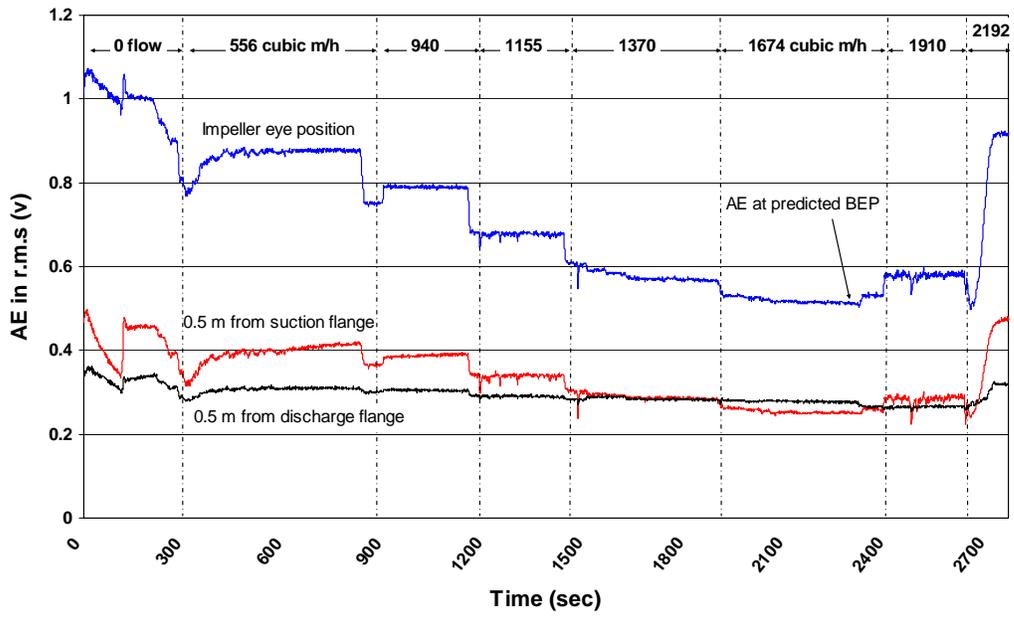
**Figure 3** AE r.m.s observations during performance test
