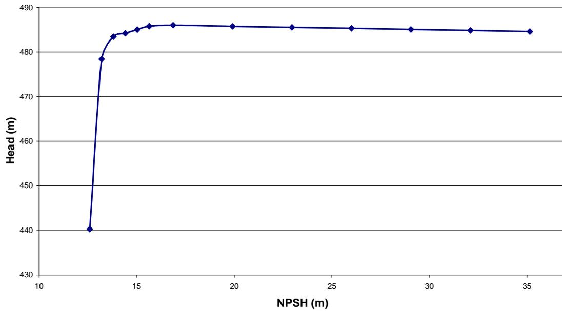
**Figure 4** Differential Head vs. NPSH at flow rate 1686 meter<sup>3</sup>/h
