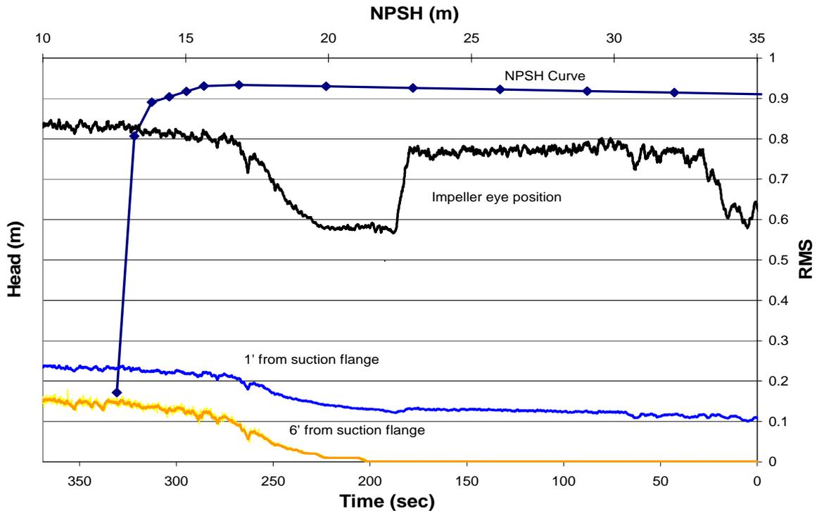
**Figure 5** AE r.m.s activity during NPSH testing
