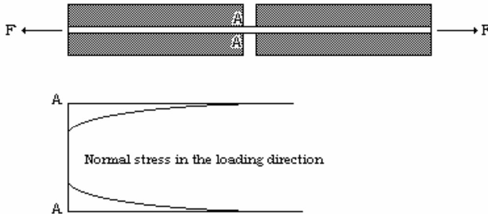
Fig. 1 Zero span test
