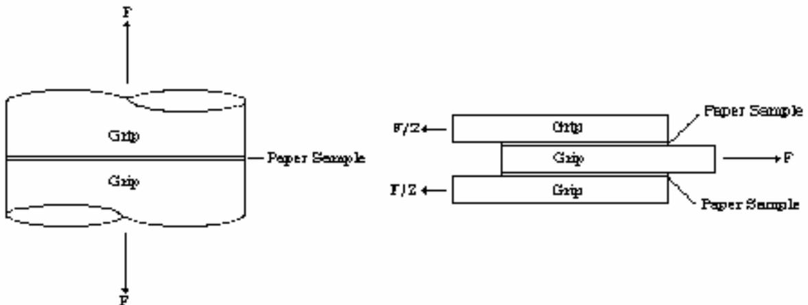
Fig. 2 Bond failure testing
