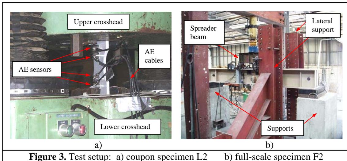
**Figure 3.** Test setup: a) coupon specimen L2      b) full-scale specimen F2
