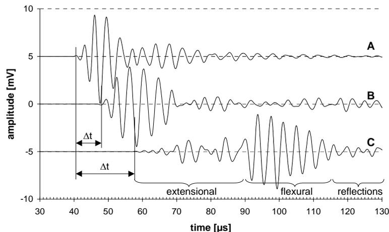
Figure 1: Acoustic waveforms to measure speed of sound. A: Sound wave from the transmitted signal; registered by directly coupling sensor P to the receiving sensor (reduced in amplitude by factor 5). B: Received signal from a 65 mm long CFC-specimen (ex-pitch orientation). C: Received signal from a 135 mm long stainless steel cylinder.
