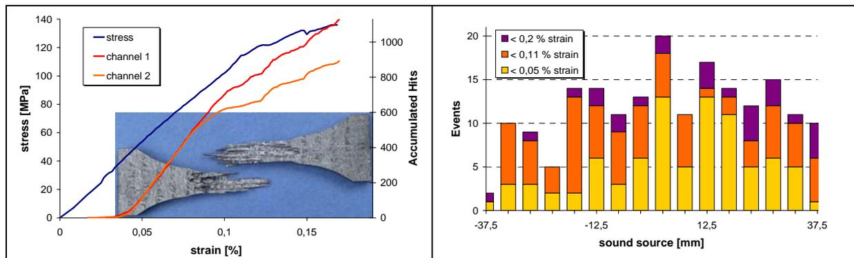
Figure 4: Tensile testing in ex-pitch (X) orientation. Left side: Stress and accumulated hits over strain + specimen after testing. Right side: Number of events over location for three different strain ranges.
