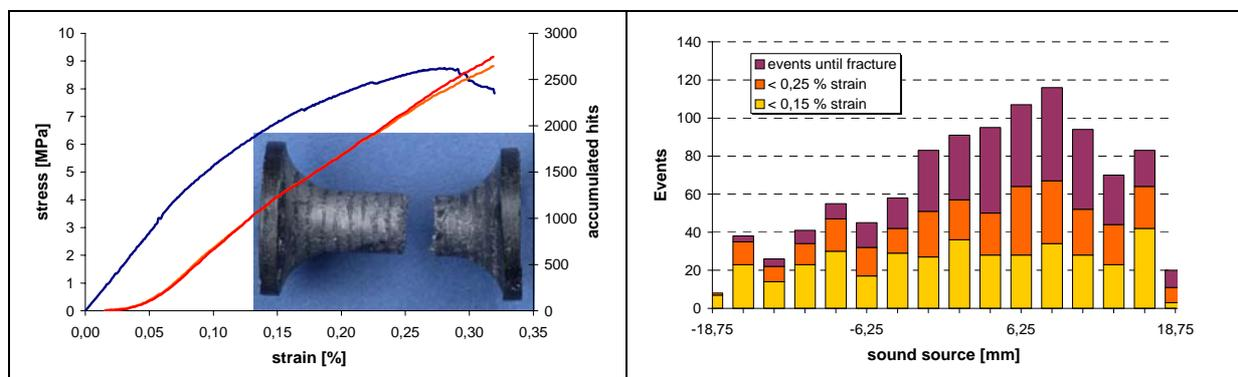
Figure 6: Tensile testing in needling (Z) orientation.
