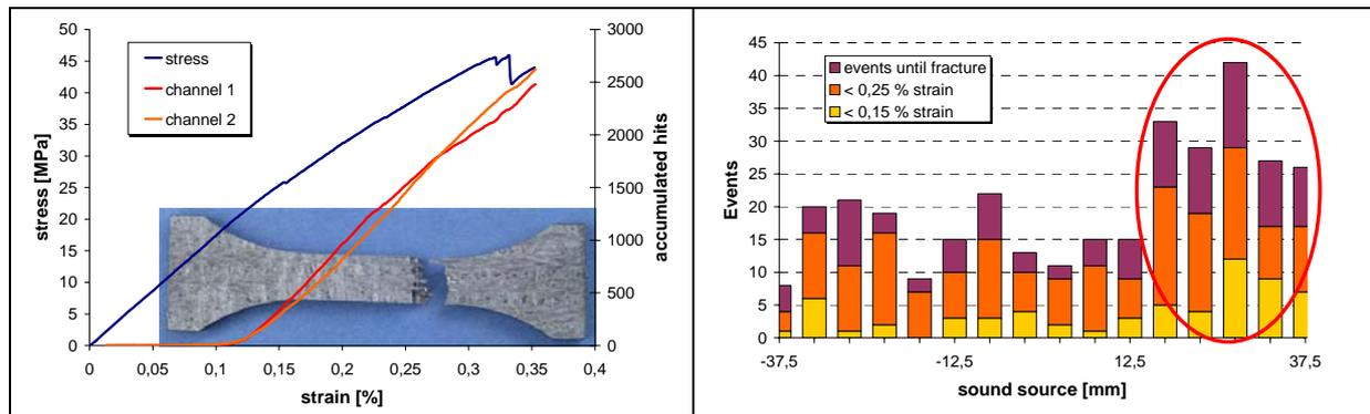
Figure 5: Tensile testing in ex-PAN (Y) orientation.
