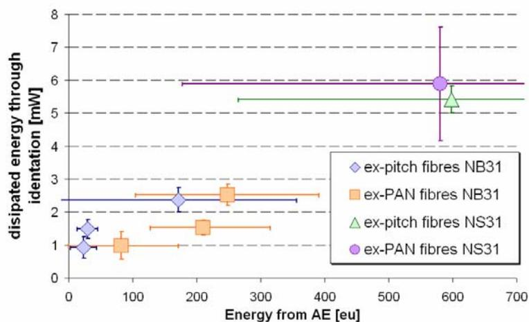
Figure 2: Correlation between mechanically dissipated energy and pseudo energy measured by AE. The error bars show the standard deviations.
