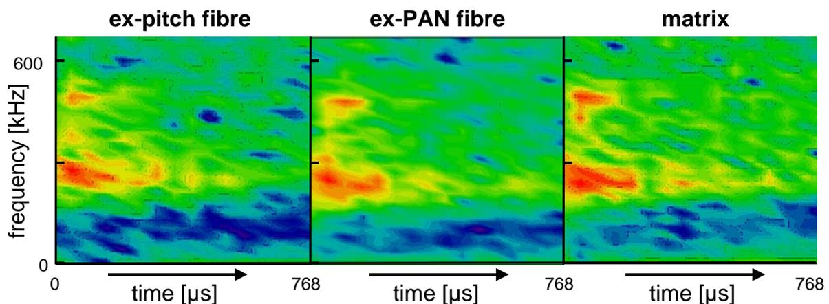
Figure 3: Normalised AE Signals obtained at the micro hardness tester at loads of 100 N analysed by windowed FFT (NB31). Small (blue) to high (red) amplitudes.
