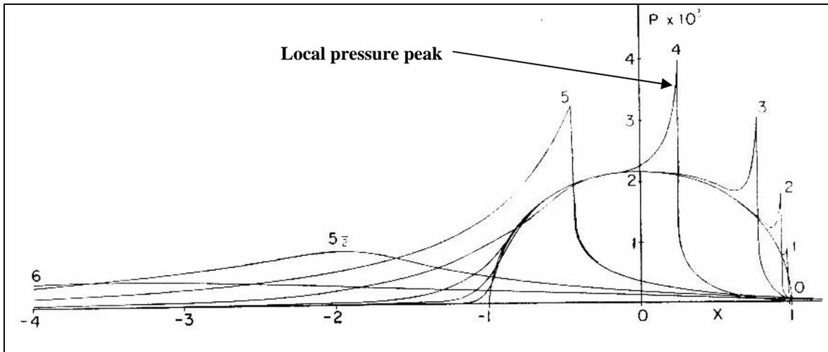
**Figure 2** Pressure distributions for a compressible lubricant with increasing speeds from plots (0) to (5) [9].
