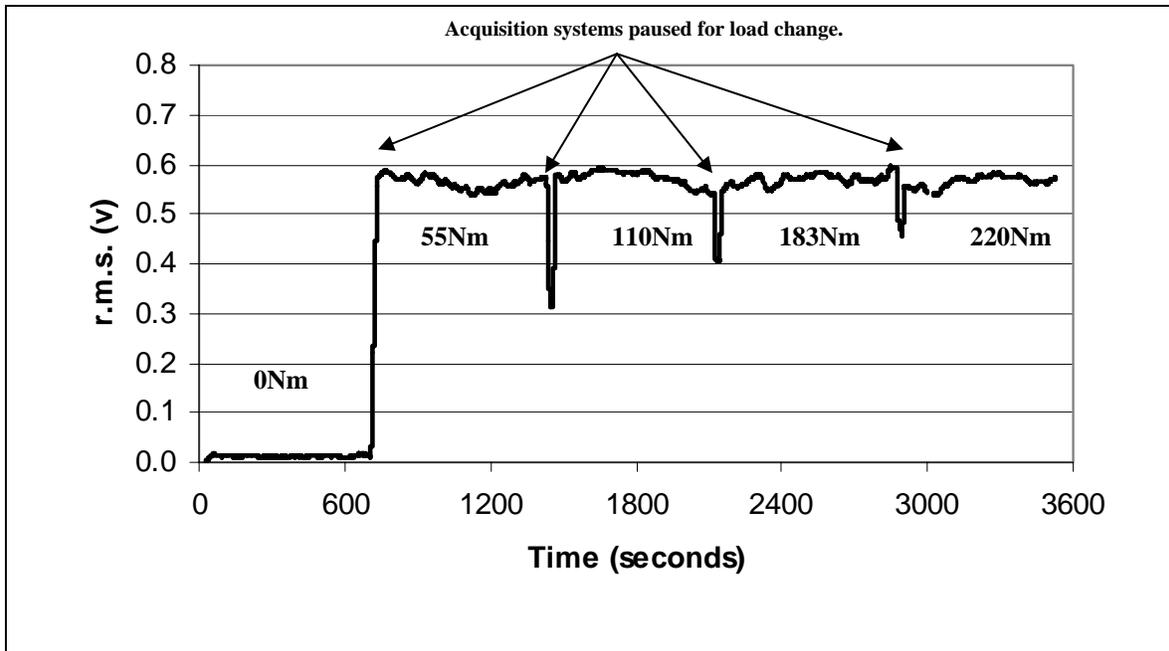
**Figure 3** AE r.m.s. remained constant with increased load at 745 rpm.
