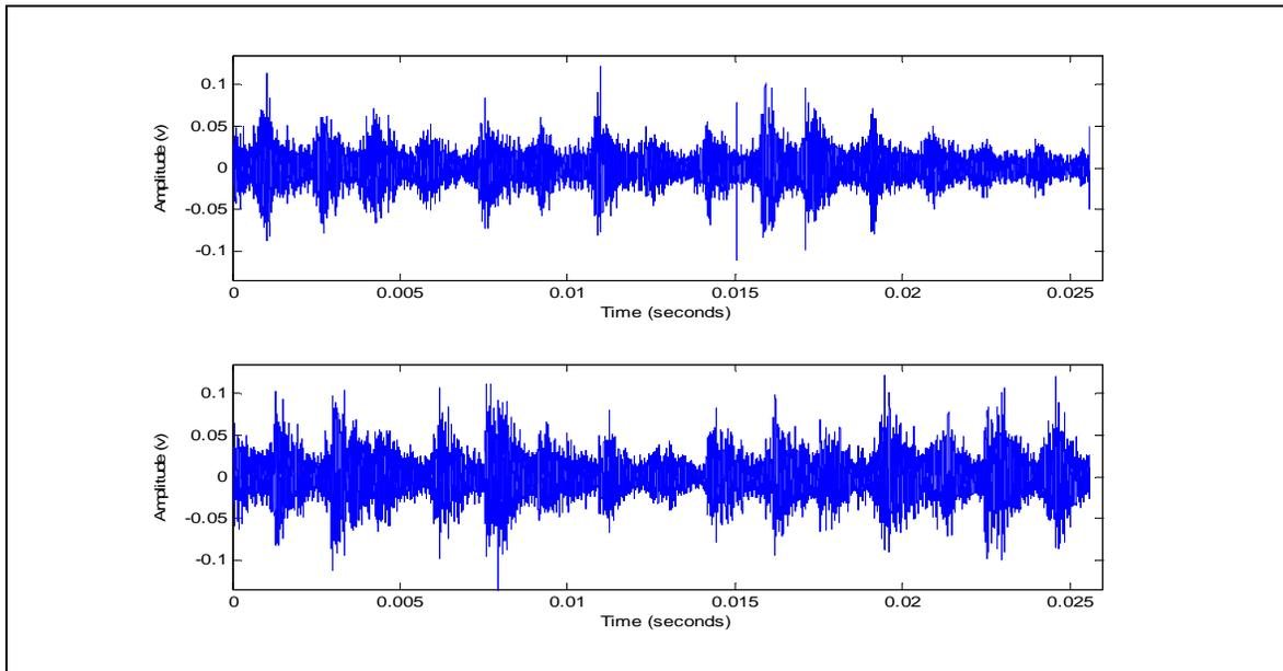
**Figure 1** Time domain of an AE signature showing clearly the AE transient response associated with gear meshing of 16 teeth for the rotational speed of 745 rpm under various loads (pre-amplification 20dB)
