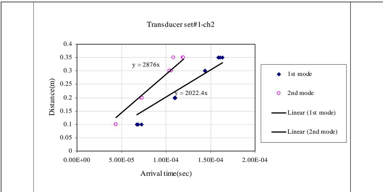
**Figure 7** Velocity changes of two modes of piston designs recorded from transducer set#1 for the second channel, piston-B3
