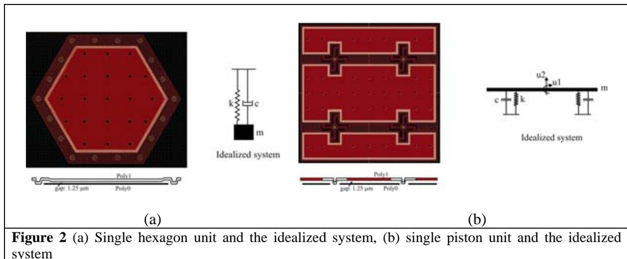
Figure 2 (a) Single hexagon unit and the idealized system, (b) single piston unit and the idealized system
