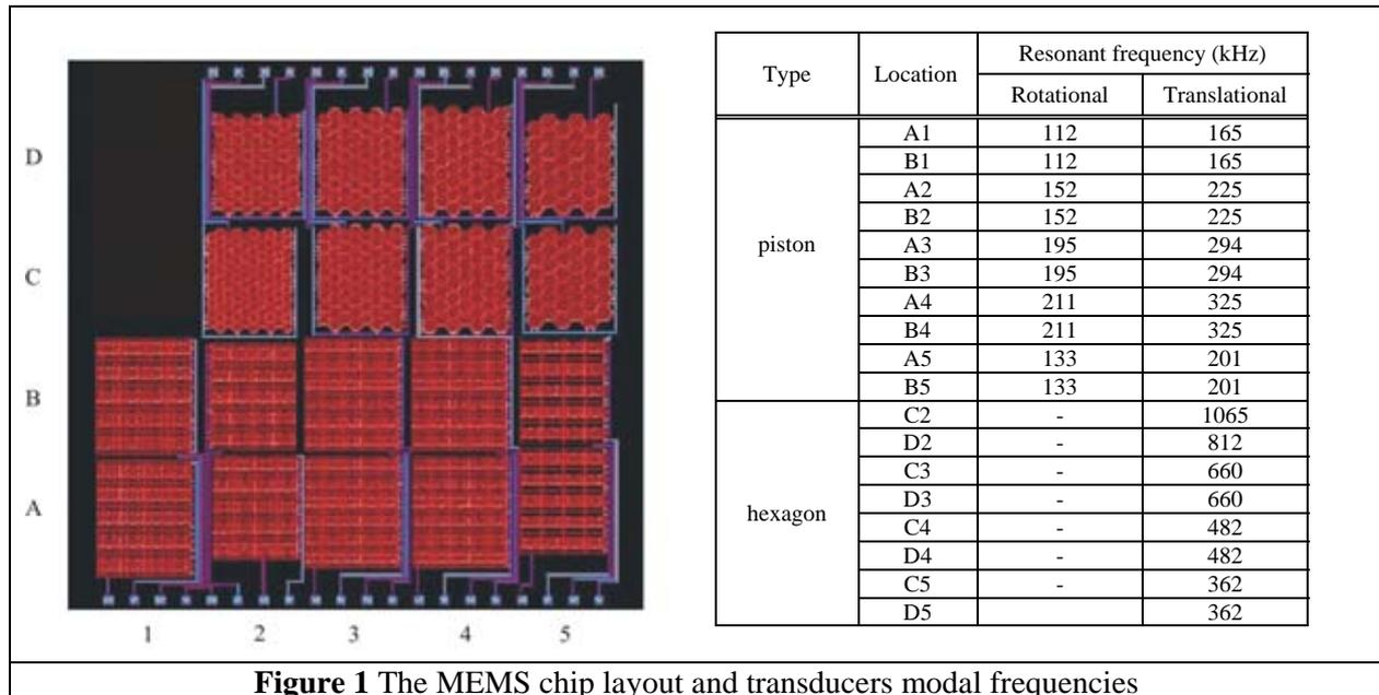
Figure 1 The MEMS chip layout and transducers modal frequencies
