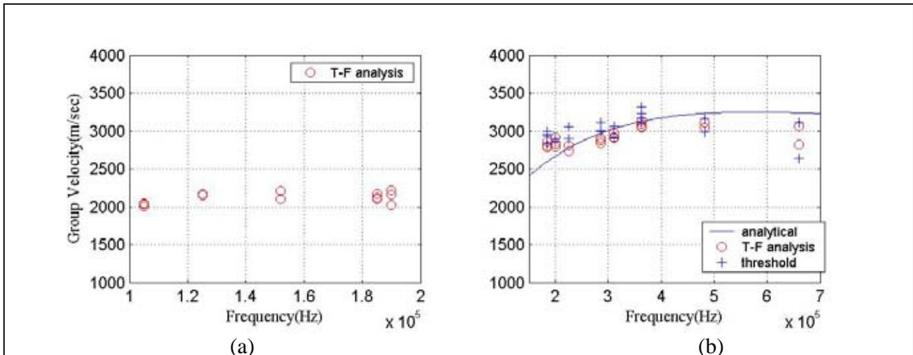
**Figure 8** (a) The velocity of the rotational mode of the piston designs, (b) the velocity of the translational mode of the piston designs and hexagon designs
