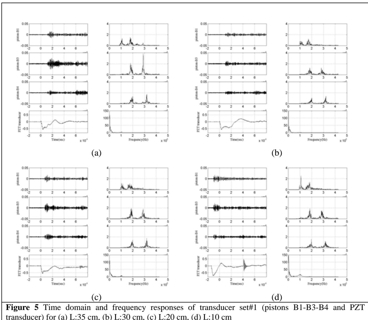
**Figure 5** Time domain and frequency responses of transducer set#1 (pistons B1-B3-B4 and PZT transducer) for (a) L:35 cm, (b) L:30 cm, (c) L:20 cm, (d) L:10 cm
