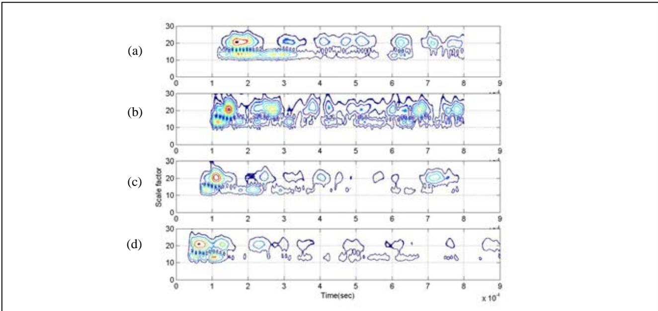
**Figure 6** Wavelet coefficients of the second channel (piston-B3) of the transducer set #1 (pistons B1-B3-B4 and PZT transducer) for four different locations, (a) L:35 cm, (b)L:30 cm, (c)L:20 cm,(d)L:10 cm
