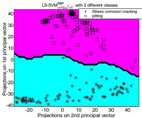
Figure 9: Decision boundary computed by the LS-SVM. In this case the LS-SVM was able to separate all SCC signals (asterisks) from the pitting signals (squares). All symbols are time series, with information compressed in 2 parameters after FFT.  $\mathbf{C}_k$ 's are represented by the data points.
