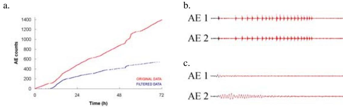
Figure 4: a. Cumulative counts of the original AE data and the “filtered” events
