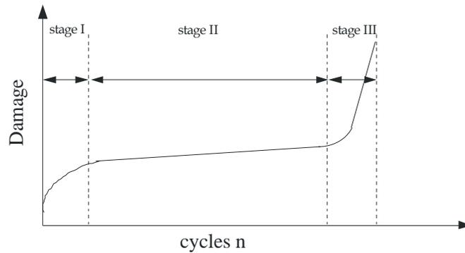
Figure 1: Typical damage development curve for quasi-isotropic composites
