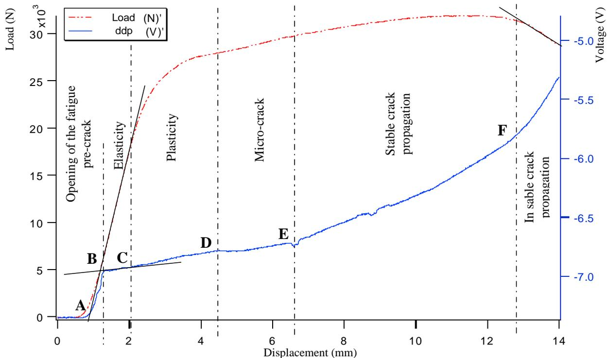
**Figure 2** Voltage is plotted along with the load versus the displacement during the tensile test of specimen C on P265GH steel.
