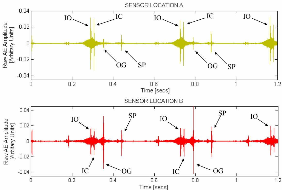
Figure 6: Typical running engine AE from sensor locations A and B with major events indicated;
