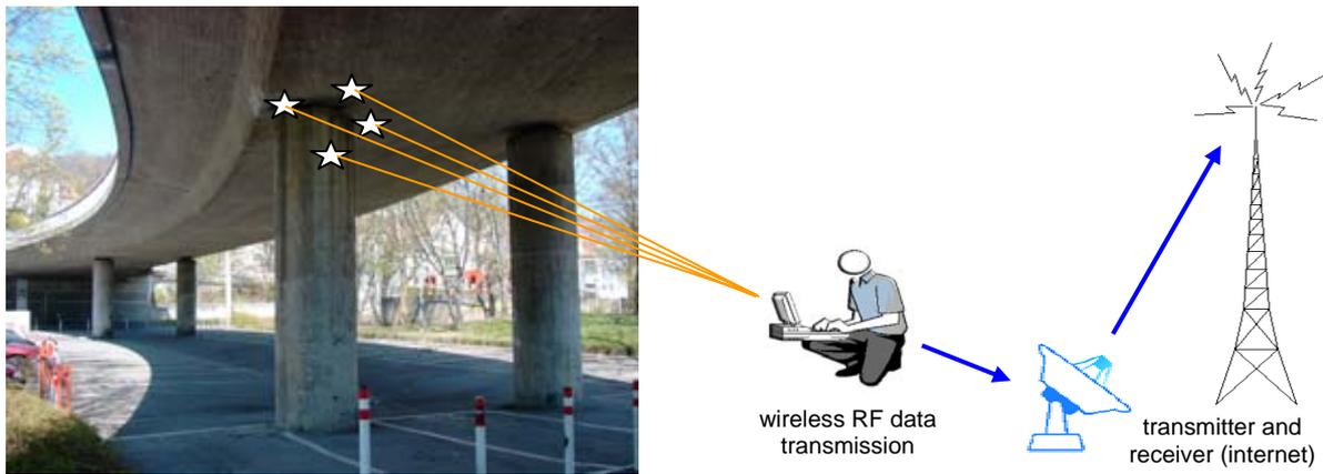
Fig. 3: Diagram of wireless sensing of large structures using radio frequency transmission technique.
