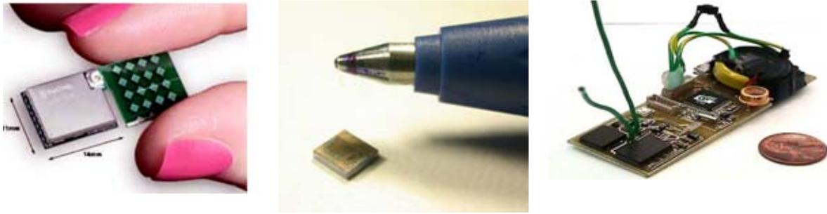
Fig. 5: Example of existing MEMS and „Motes“(courtesy of UC Berkeley).
