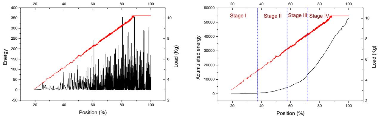
Figure 2. AE results for Scratch 1, Sample E (TiN). Left: Energy of hits and load vs. position %. Right: accumulated energy vs. position %.
