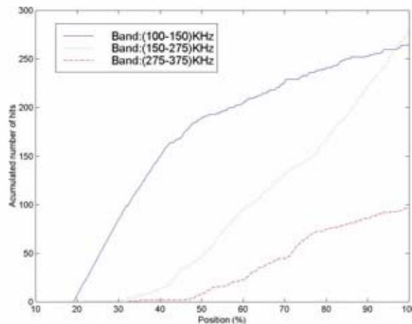
Figure 6. Accumulated number of hits vs. Position (%) for the different frequency bands.
