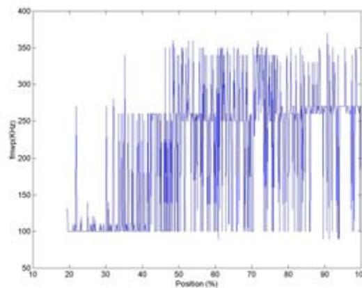
Figure 4. Frequency at which WP is a maximum ( $f_{MWP}$ ) vs. position %. Scratch 1, Sample E (TiN).
