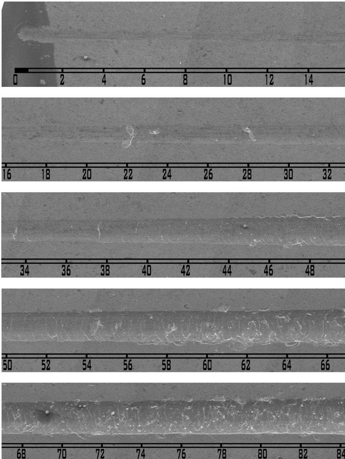
Figure 1. Scanning electron micrograph. Scratch 1, Sample E, TiN.
