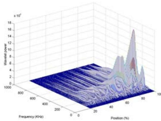
Figure 3. Wavelet power vs. frequency and position %. Scratch 1, Sample E (TiN).
