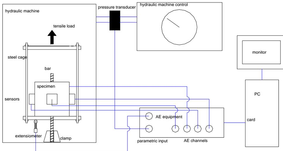
Figure 1: Diagram of the pull-out experiment with AE.
