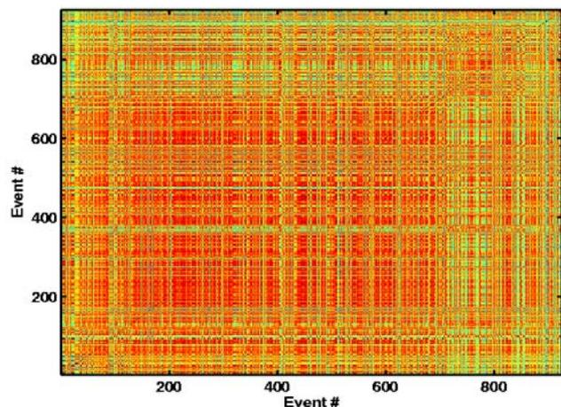
The similarity matrix in Fig. 3 does not show very significant colour contrasts between the 3 major fracture periods. To check the significance of these 3 major clusters, a principal component analysis was performed. Herefore, the raw signals were taken, eigenvectors
