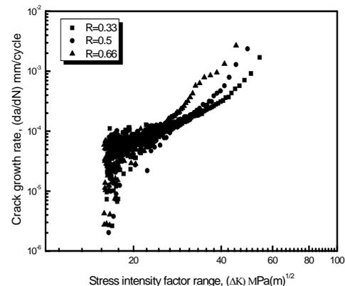
Fig. 3 Relation of crack growth rate and stress intensity factor range
