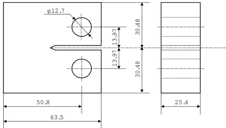
Fig. 1 Configuration of Specimen
