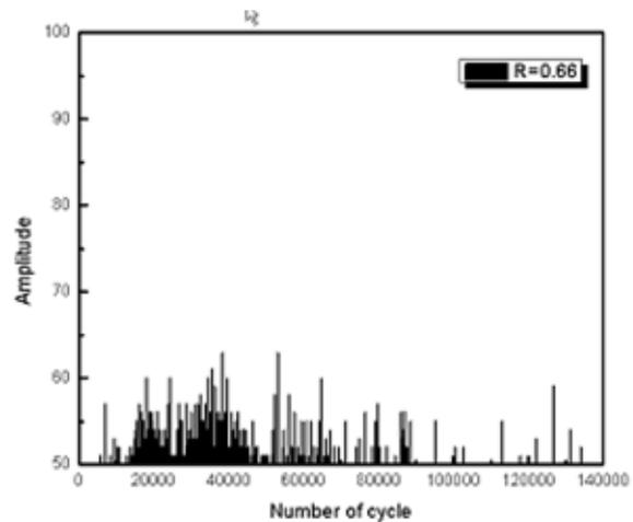
Fig. 11 Relation of amplitude and number of cycles for R=0.66
