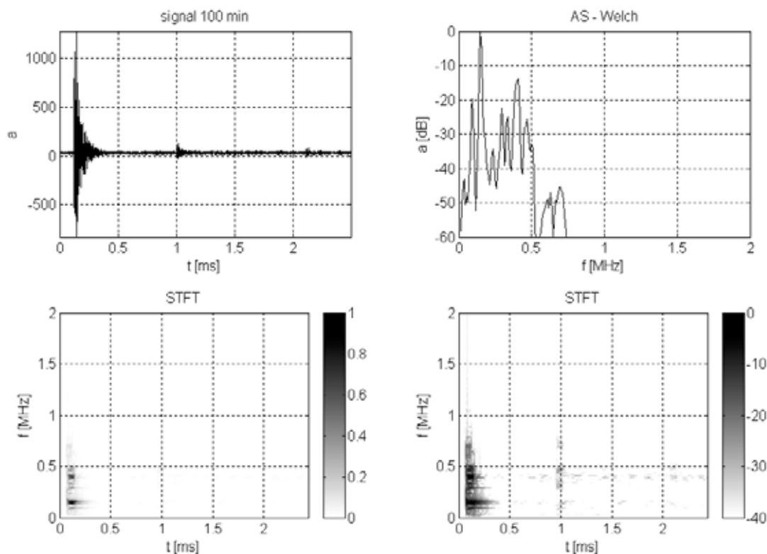
Fig 10 Exemple of AE events with frequency spectrum and Short Time Fourier Transformation – low alloy steel (time 100 min.)
