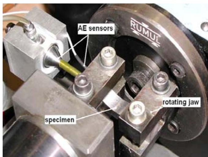
*Fig.1 Arrangement of AE tests on electro-resonance testing machine*
