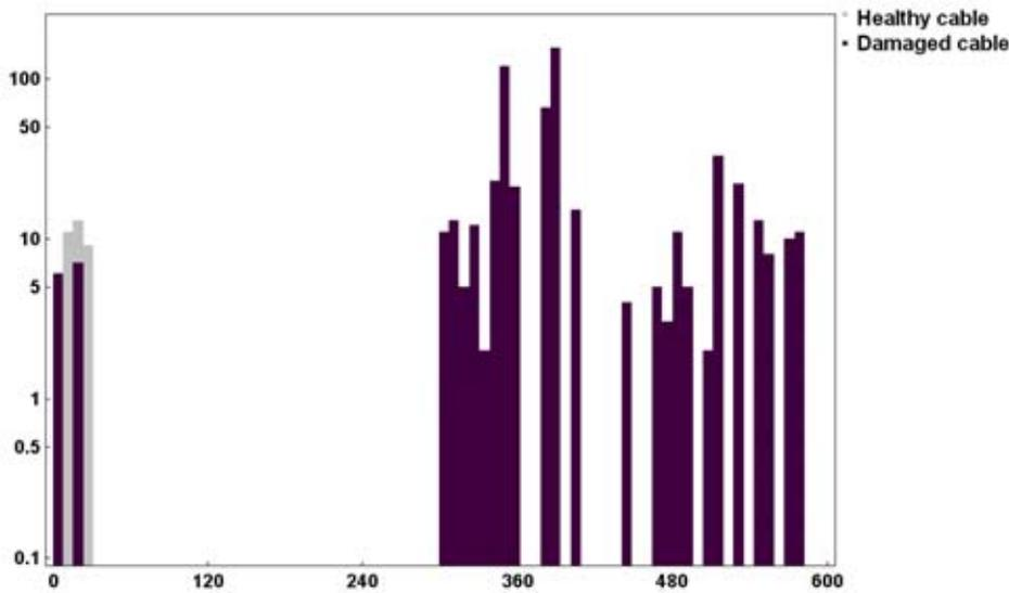
Figure 6 : Frequency distribution of AE counts in the presence of defects or not under clamp.
