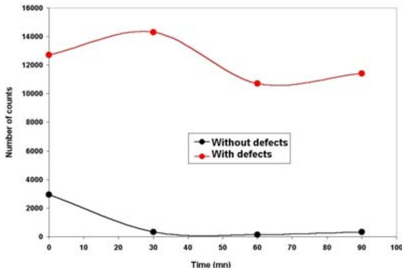
Figure 2 : Evolution of the number of AE counts versus time in the presence of defects or not on cable.
