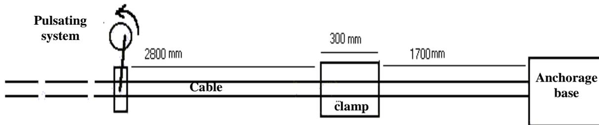
Figure 1 : Rope test set-up with a cable put in place.
