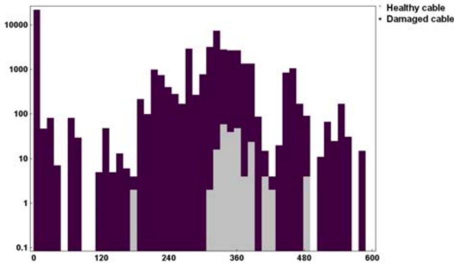
Figure 5 : Frequency distribution of AE counts in the presence of defects or not under base anchoring.
