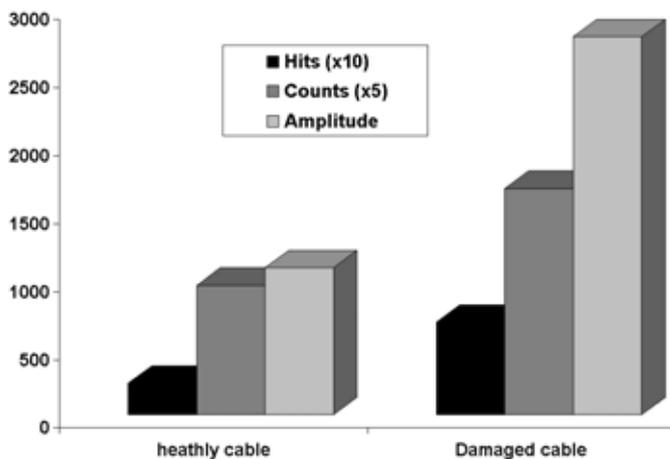
Figure 4 : Acoustic emission activity according to the presence or not of defects on the cable under collar.
