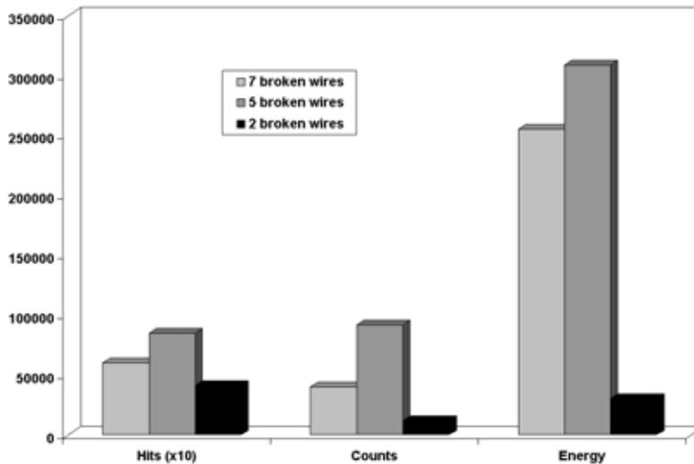
Figure 7 : AE activity for three degree of degradation under base anchoring of a multilayer cable
