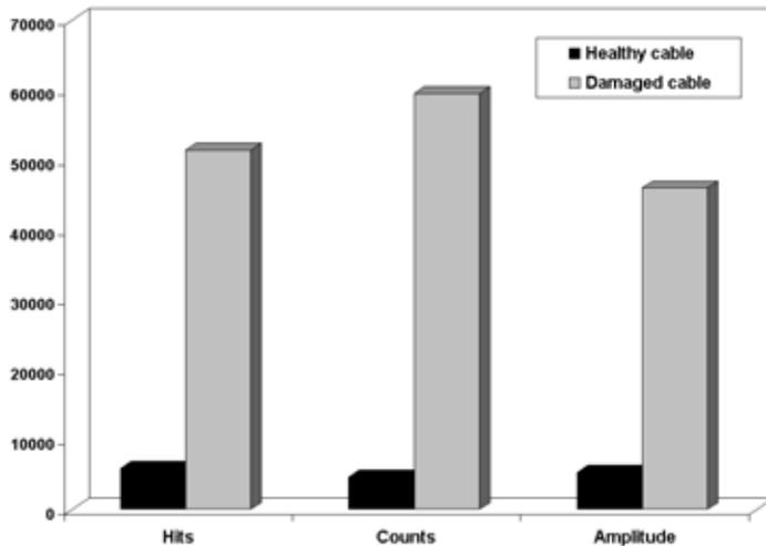
Figure 3 : Acoustic emission activity according to the presence or not of defects on the cable under base.
