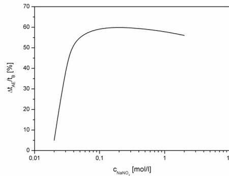
**Fig. 4** Relation between the time of AE activity and the fracture time over the concentration of  $\text{NaNO}_2$
