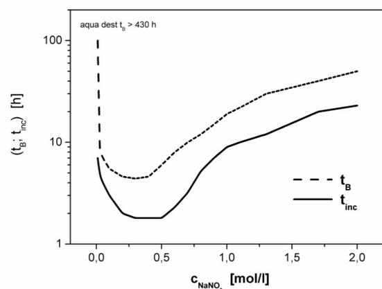
**Fig. 2** Dependence of the time of fracture and the time of AE activity on the concentration of  $\text{NaNO}_2$  during a CLT of CuZn37
