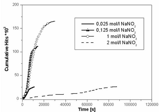
**Fig. 6** Cumulative hits of AE signals during a CLT for CuZn37 in different concentrations of  $\text{NaNO}_2$
