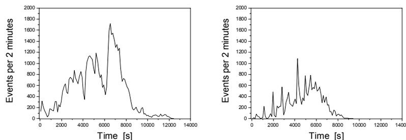
**Fig. 9 Comparison of the distribution of the AE events during a CLT in 0.25 mol/l NaNO<sub>2</sub> without (left) and with (right) an addition of 0.001 % BTA – blend starting after the incubation time**
