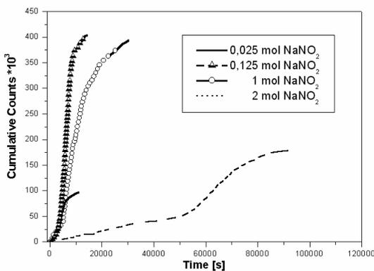
**Fig. 5** Cumulative counts of AE signals during a CLT for CuZn37 in different concentrations of  $\text{NaNO}_2$
