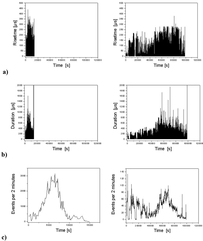
**Fig. 7 Comparison of the AE parameters risetime (a), duration (b) and the distribution of the AE events (c) of a CLT between 0.125 mol/l NaNO<sub>2</sub> (left) and 2 mol/l NaNO<sub>2</sub> (right) starting after the incubation time**
