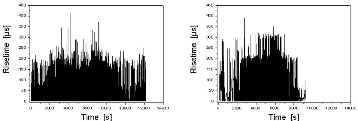
**Fig. 8 Comparison of the risetime during a CLT in 0.25 mol/l NaNO<sub>2</sub> without (left) and with (right) an addition of 0.001 % BTA – blend starting after the incubation time**
