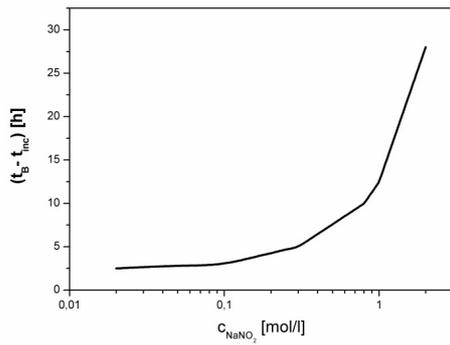
**Fig. 3** Time of enhanced AE activity in correspondence of the concentration of  $\text{NaNO}_2$  during a CLT of CuZn37
