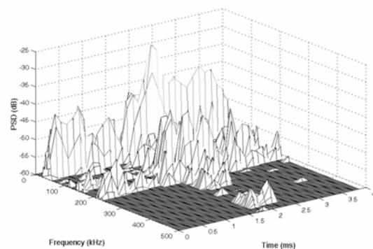
Figure 10: Three-dimensional spectrogram of amplitude spectrum calculated for AE pulses generated by electrical discharges in the point-plane system in air, during the negative voltage half-period
