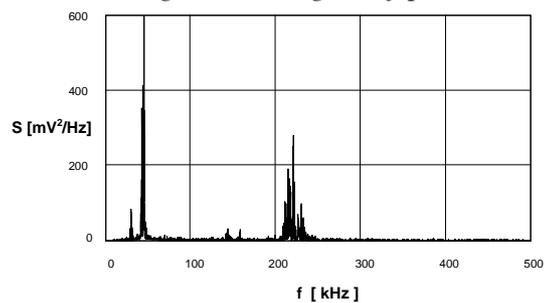
Figure 4: Energy density spectrum run of the AE pulses generated by electrical discharges in the point-plane system in air, during the negative positive voltage half-period
