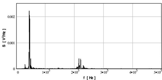
Figure 2: Energy density spectrum run of the AE pulses generated by electrical discharges in the point-plane system in air, during the positive voltage half-period
