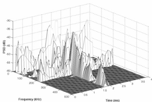
Figure 7: Three-dimensional spectrogram of amplitude spectrum calculated for AE pulses generated by electrical discharges in the point-plane system in air, during the positive voltage half-period
