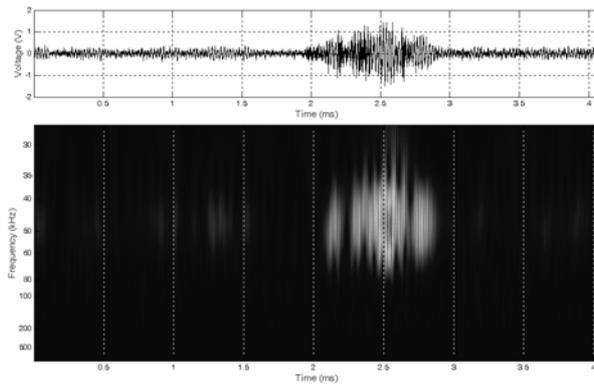
Figure 11: CWT of the AE pulses generated by electrical discharges in the point-plane system in air, during the positive voltage half-period
