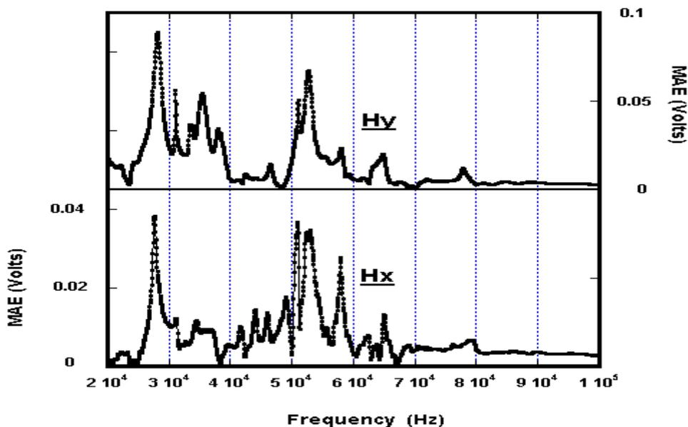
**Figure 3.** Comparison of MAE signals obtained by applying the magnetic field both along the axis of the Metglas ribbon ( $H_x$ ) and in a perpendicular direction ( $H_y$ )
