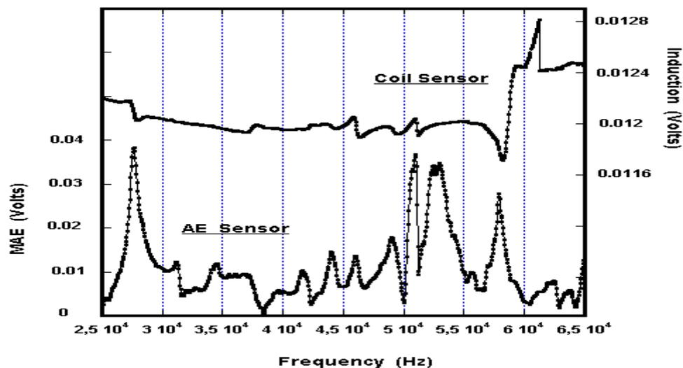
**Figure 2.** Magnetoelastic resonances in a Metglas ribbon obtained from a coil and AE sensors using Lock-in amplifiers.
