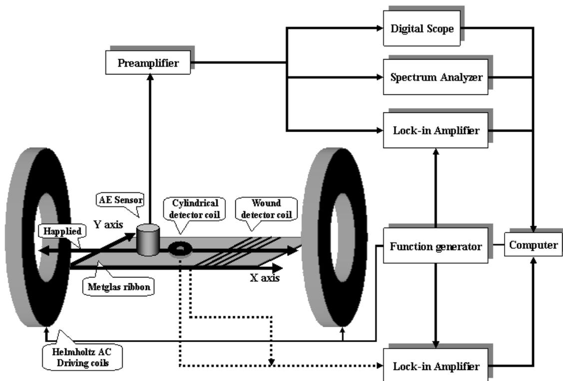
**Figure 1.** Experimental device for the simultaneous measurement of magnetoelastic resonances using AE and induction sensors.
