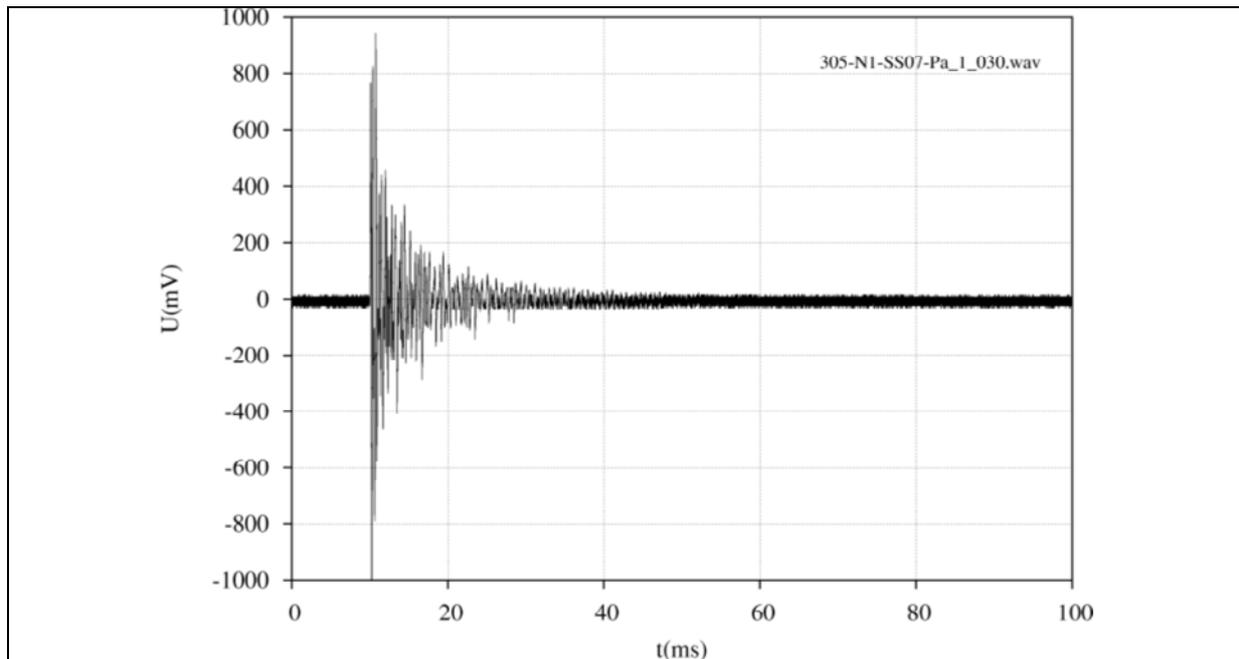
Fig.3 Time-domain response record for a roofing tile No.5 after one -70°C degradation test cycles.
