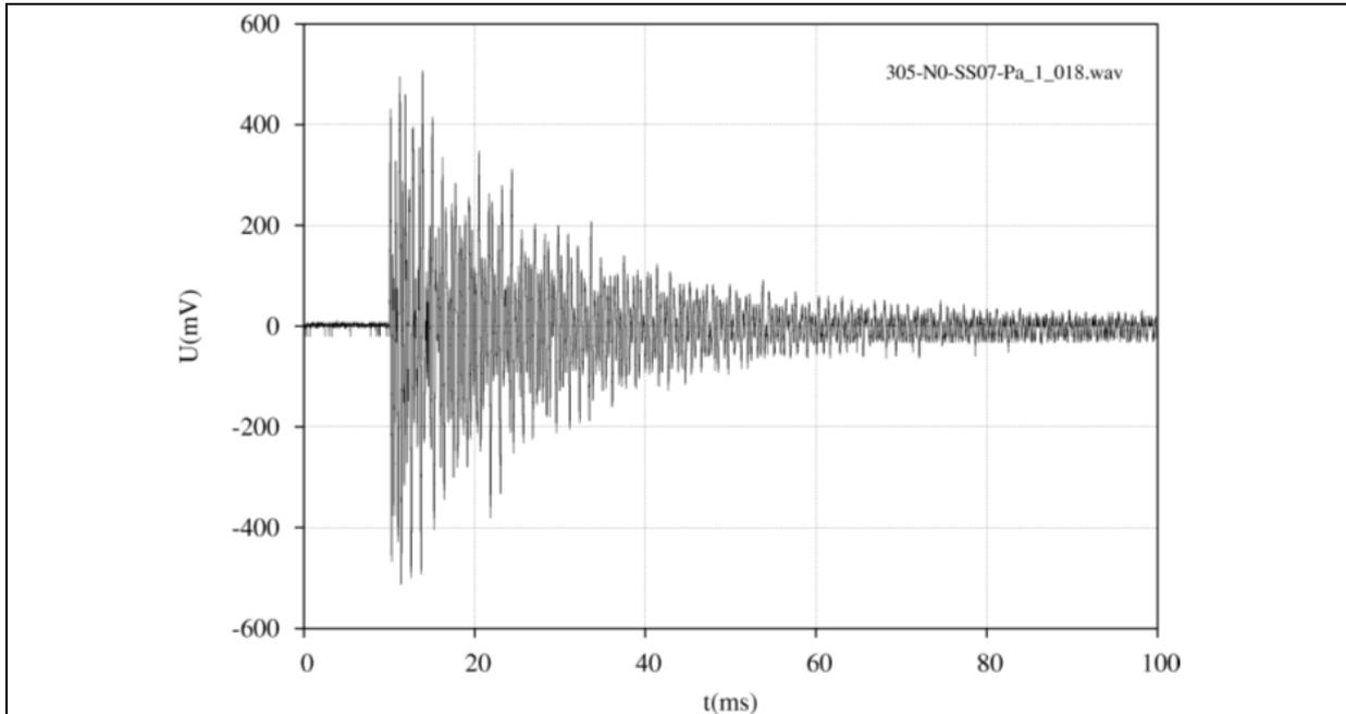
Fig.1 Time-domain response record for a roofing tile No.5, which had been fabricated using an old technology. Measurement was made before degradation.
