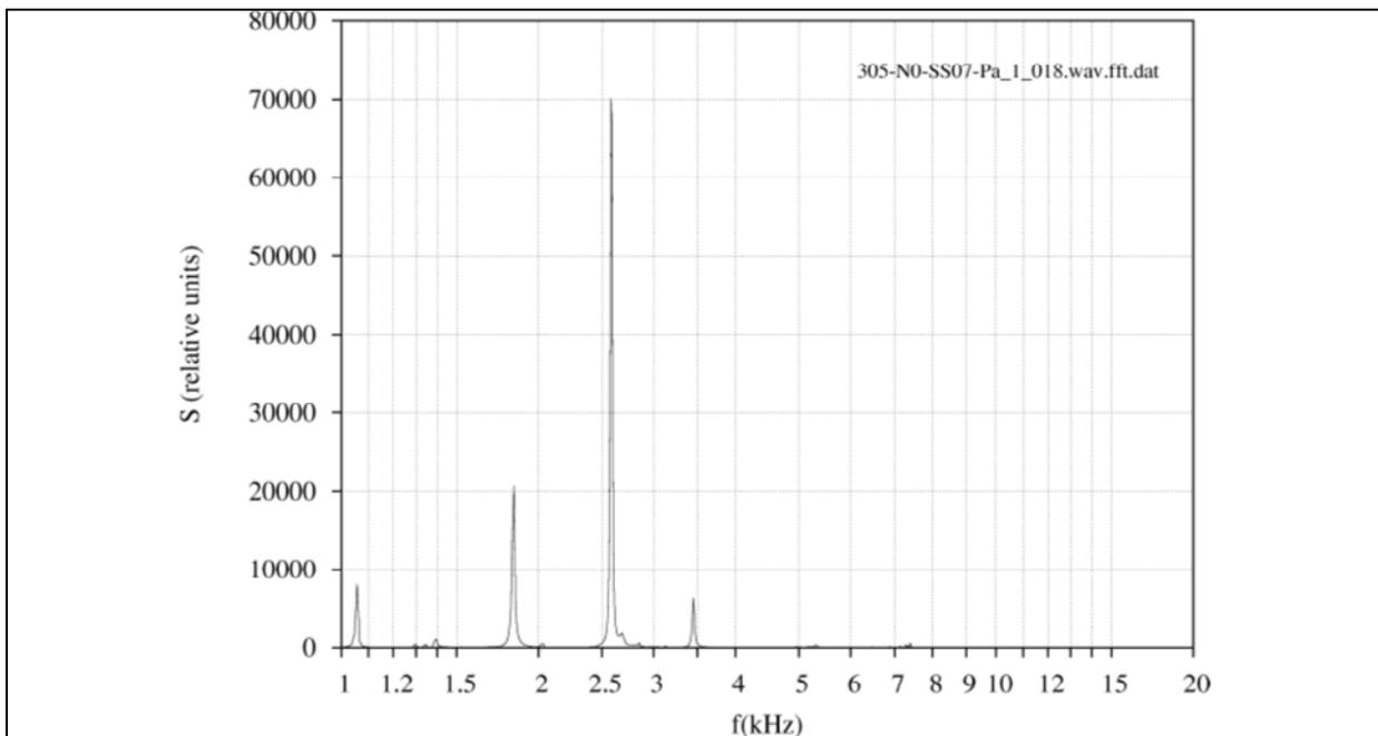
Fig.2 The power spectral density versus frequency plot for specimen No.5, which had been fabricated using an old technology. Measurement was made before degradation.
