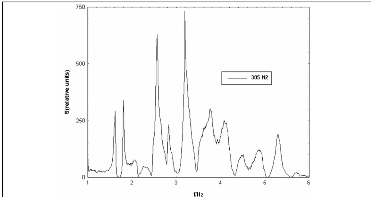
Fig.5 The power spectral density versus frequency plot for specimen No.5 after two -70°C degradation test cycles.
