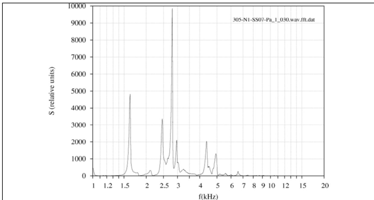
Fig.4 The power spectral density versus frequency plot for specimen No.5 after one -70°C degradation test cycles.
