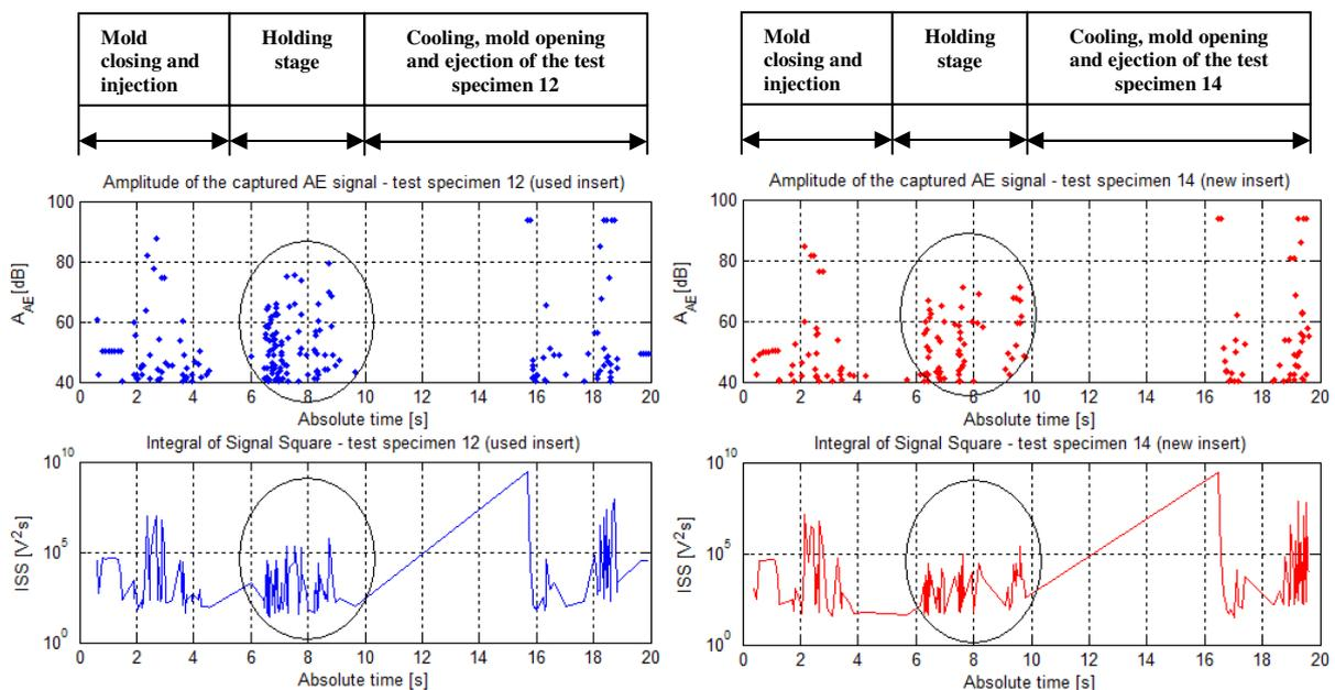
Fig.8. Captured AE signals for test specimen 12 and 14 inside one production cycle
