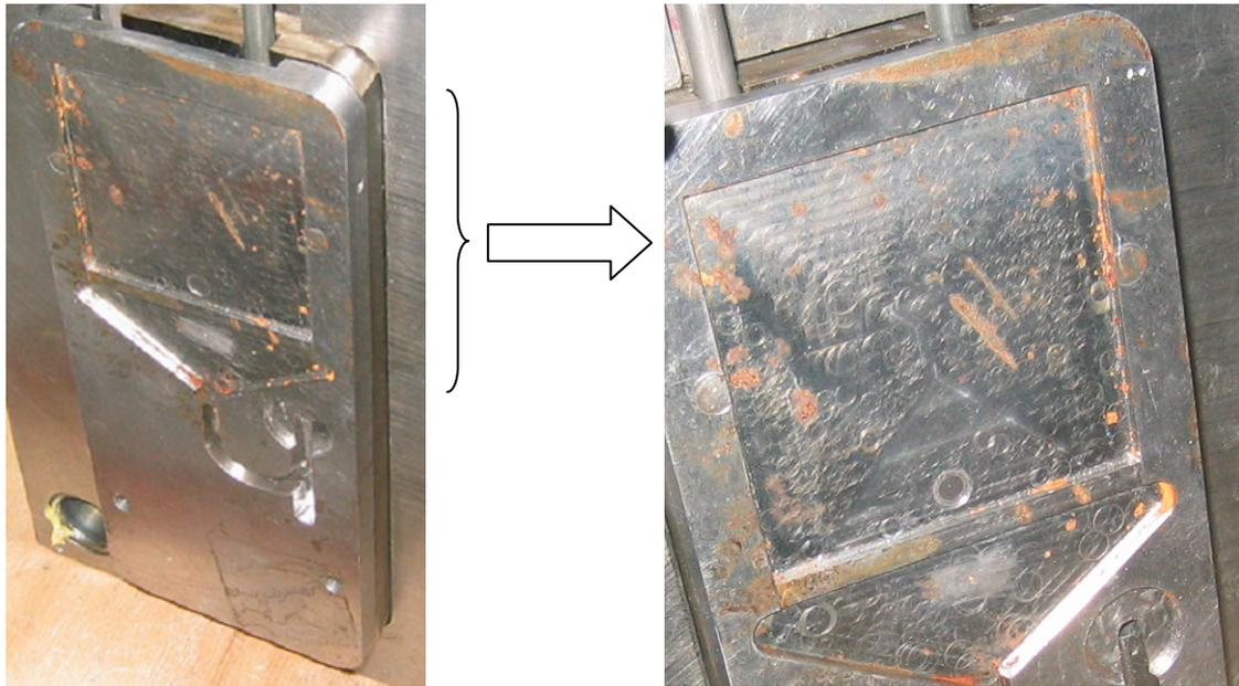
Fig.4. A closer look on the (corroded) injection mold engraving insert's front side.
