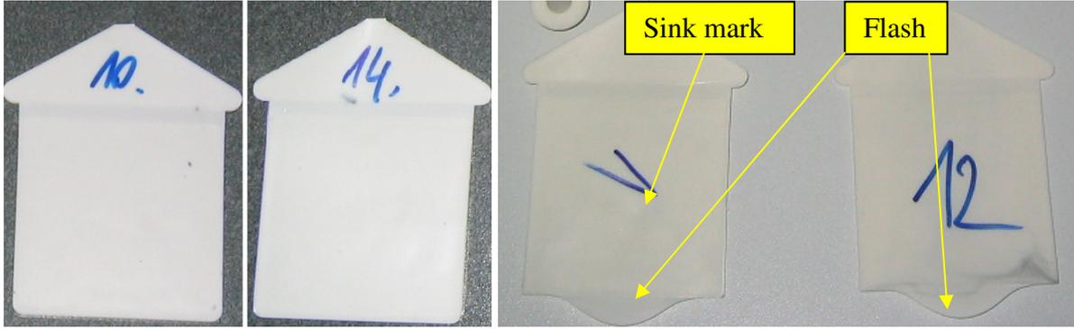
Fig.5. Specimens produced with unused (10 and 14) and corroded (1 and 12) injection mold engraving insert.
