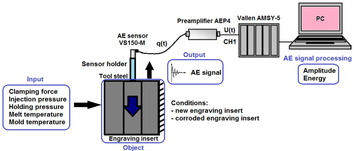
Fig.1. Diagram of the experimental setup.
