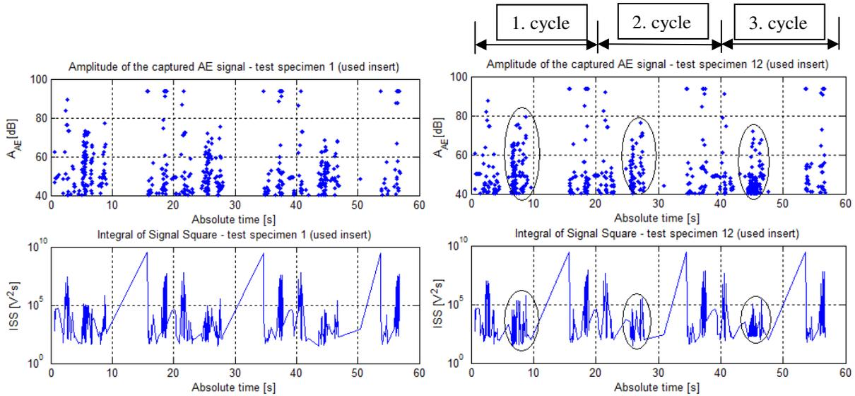
Fig.6. Captured AE signals for test specimen 1 and 12 on a used injection mold insert
