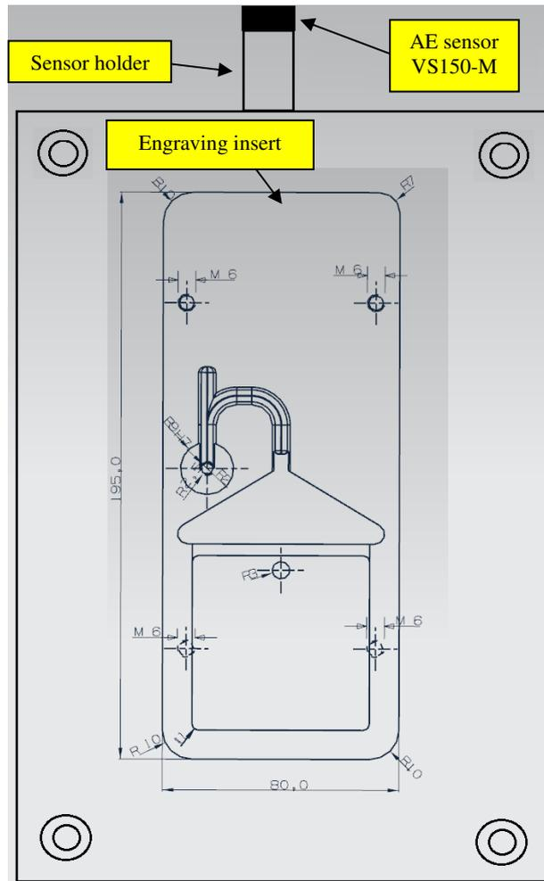
Fig.2. Schematic drawing of the mold's ejection side.
