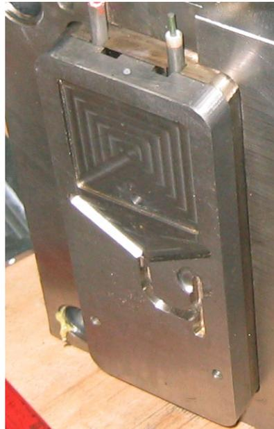
Fig.3. Unused injection mold engraving insert
