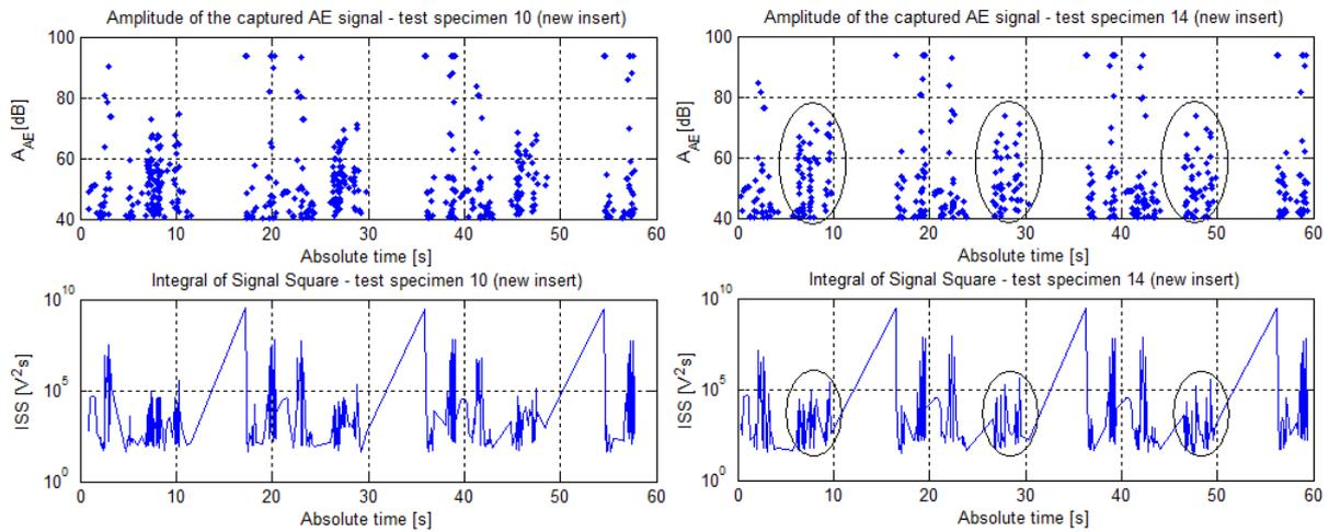
Fig.7. Captured AE signals for test specimen 10 and 14 on a new injection mold insert
