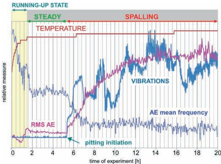
Figure 4. Observation of test: AE, vibration, temperature
