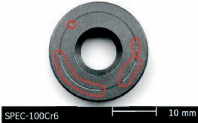
Figure 6. Surface damage after test on material specimen
