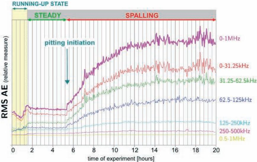
Figure 5. RMS AE – frequency distribution
