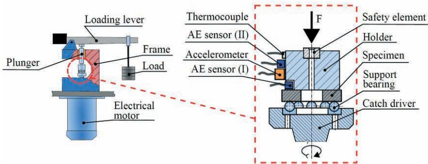
Figure 1. Experimental test-rig layout [1]
