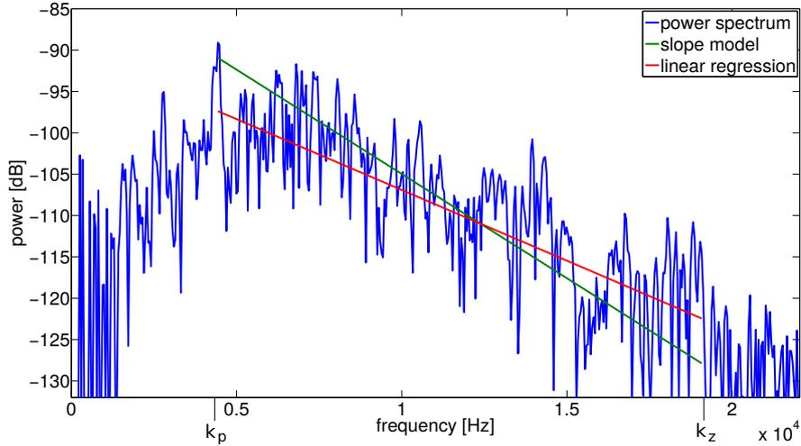
Figure 2 : Power spectrum of a cracking sound in the first part of the impulse.
