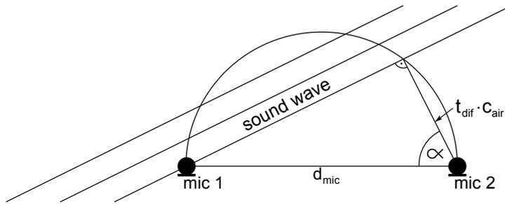
Figure 4 : Principle drawing for the localisation.
