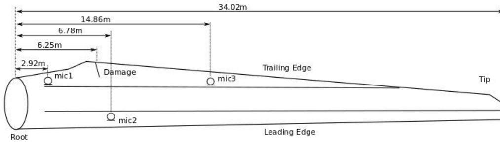
**Figure 2. Principle drawing of the rotor blade measurements set-up of the fatigue test. At 6.25m the trailing edge crack occurred.**
