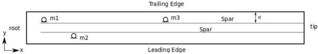
**Figure 1. Principle drawing of the rectangular representation of the rotor blade**
