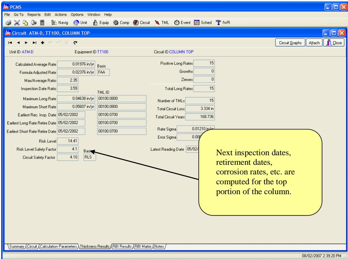
Figure 1: Calculated Values for Circuit Corrosion
