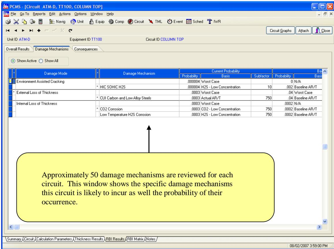
Figure 5: Likely Damage Mechanisms for a given Circuit
