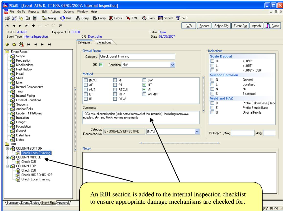
Figure 9: Internal Inspection Checklist with RBI Checking
