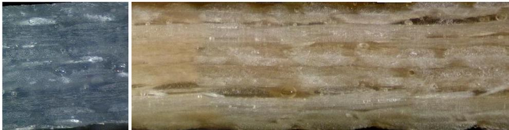
Figure 2 Side view through the thickness of composite plate before, left and right after immersion in water at 65° C for 24 months. The change of colour of the resin is one of the changes after immersion. Extensive cracks can be seen on the exposed specimen. The thickness of the pictured plate material is 3.84 mm.
