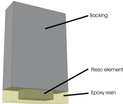
Figure 6 Schematic diagram of the constructed transducer
