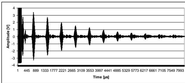
Figure 11 A-Scan obtained using single sided 4 transducers array
