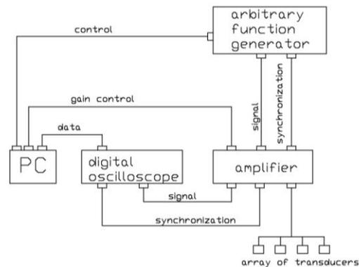
Figure 5. Equipment set-up
