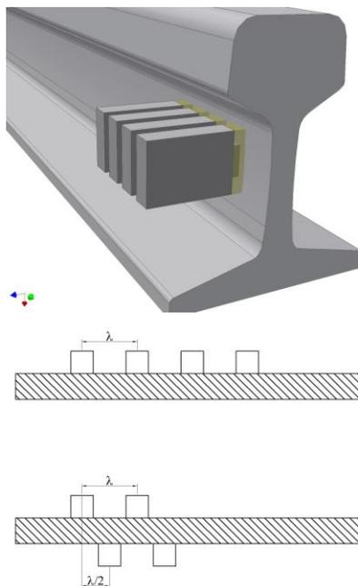
Figure 7. Transducers arrangement
