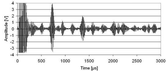
Figure 13. A-Scan from specimen containing defect
