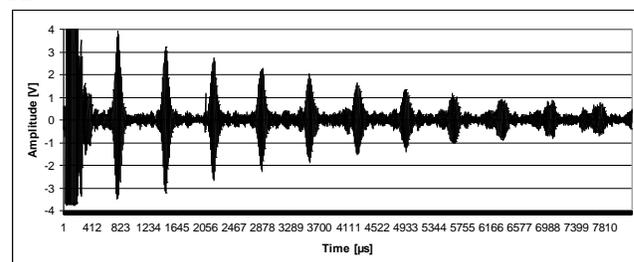
Figure 9 Mode T2 in the web of the rail using single transducer at 70 kHz
