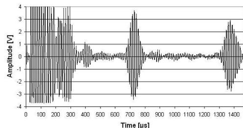
Figure 14. A-Scan of specimen containing alumino-thermic weld
