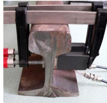
Figure 8. Clamping of the transducers
