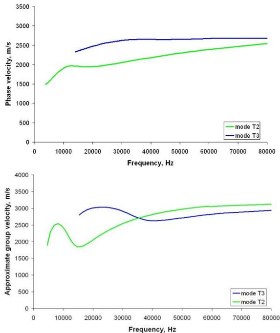
Figure 3 Dispersion curves for rail type S49
