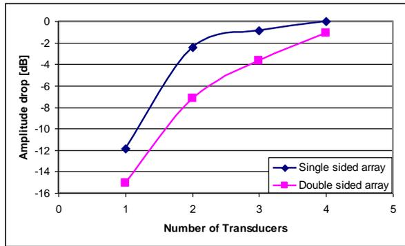
Figure 10 Amplitude of the back-wall echo for different transducer arrays
