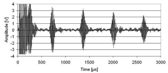
Figure 12. A-Scan from defect free specimen
