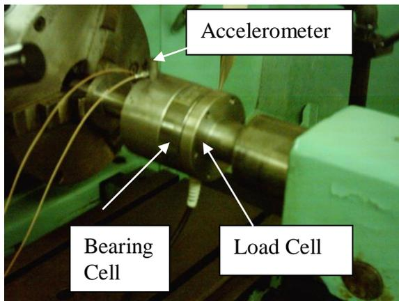
Figure 2: Accelerometer and Load cell sensor
