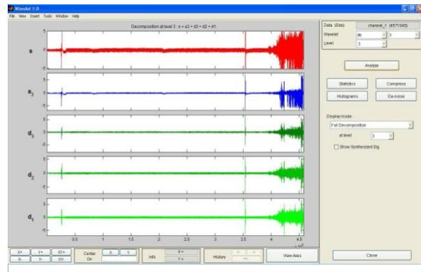
Figure 9. Wavelet db 3 (level of analysis 3)
