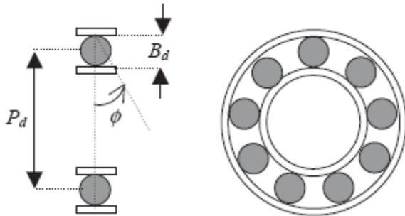
Figure 5. Ball Bearing
