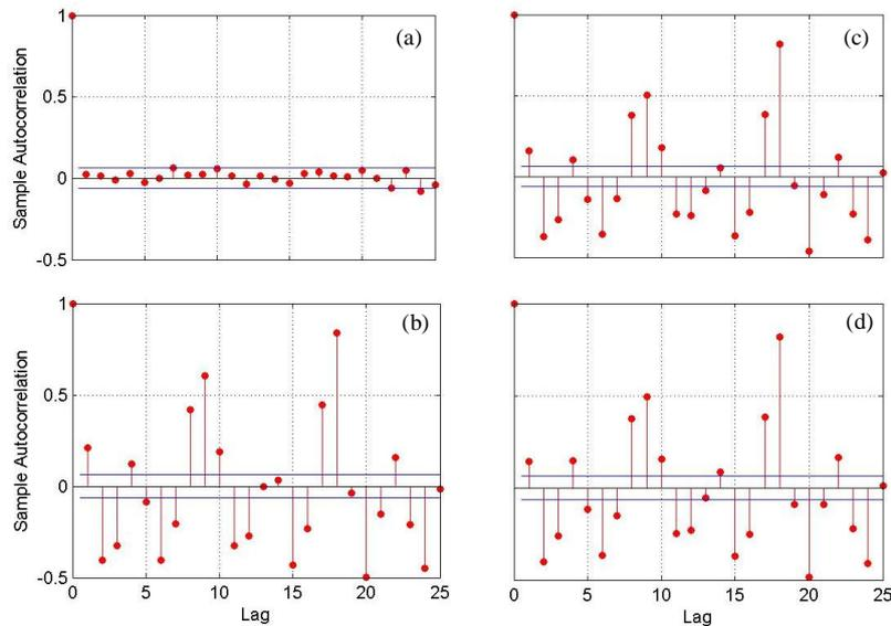
Figure 6: Autocorrelation coefficients of residuals  $e[t]$  from test runs with system (a) in healthy state, (b) with one hole, (c) with two holes and (d) with three holes (horizontal lines designate statistical limits at the  $\alpha=10^{-5}$  risk level)
