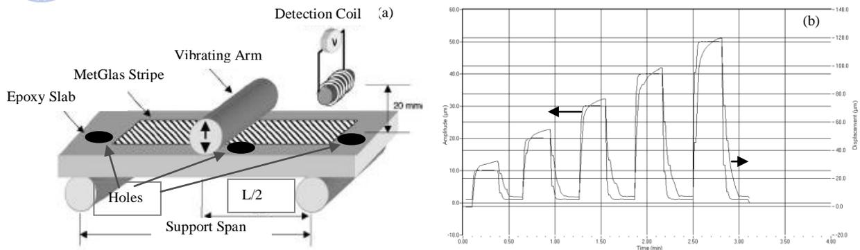
Figure 1: (a) Schematic of the experimental set up with the black spots indicating the inflicted damage locations (holes of diameter equal to 2.25mm); (b) DMA dynamic loading chart with the vibration amplitude (left y-axis) and the slab response (displacement, right y-axis) versus time.
