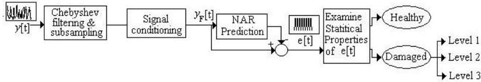
Figure 2: Operational principle of the damage diagnosis scheme
