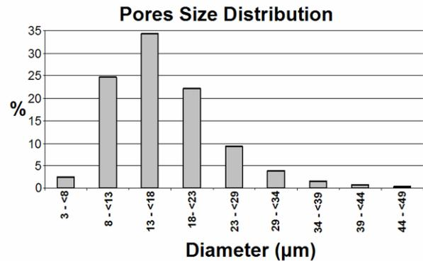
Figure 4: Pore size distribution calculated with the sphere fitting method of Hildebrand and Ruegsegger [6]
