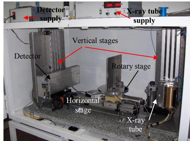
Figure 1. Picture of the CT/DR system prototype developed at the USC.
