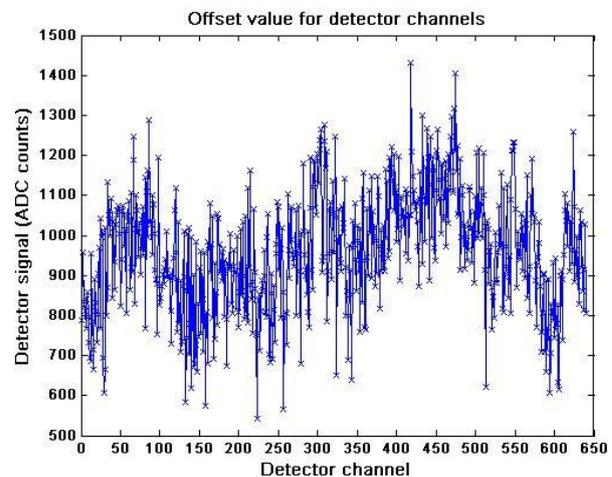
Figure 5. Detector offset variations between channels (raw data).
