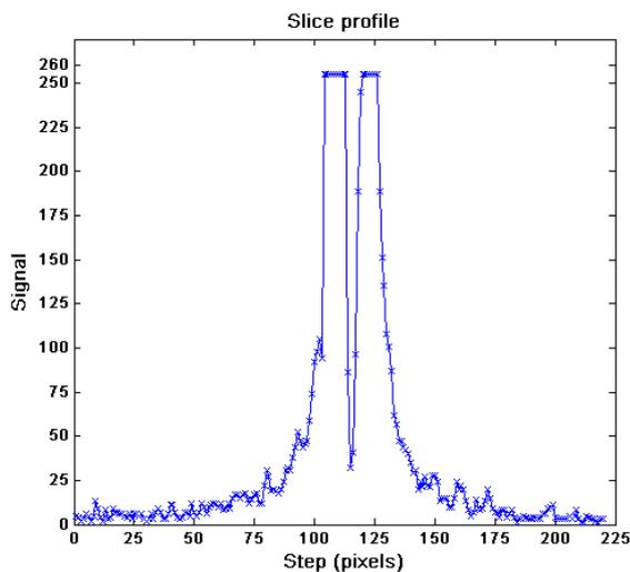
Figure 10c. Slice profile, showing the signal difference for the welding pore.
