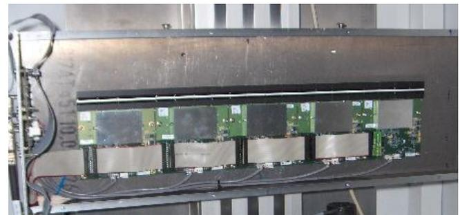
Figure 2. Radiation detector system. A 512 mm long linear array is shown made of 5 readout modules with 8 x 32 detection elements (0.8 mm pitch) per module.
