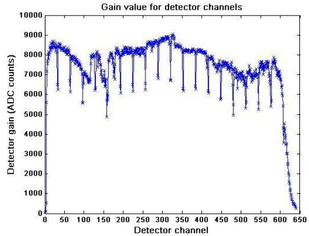
Figure 4. Flat field detector response variations between channels (raw data).
