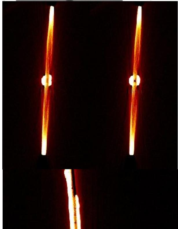
Figure 10a. Radiograph of a MIG weld on two aluminium plates (up). Details on two slices of the weld extracted from the 3D data set and a frontal view (down).
