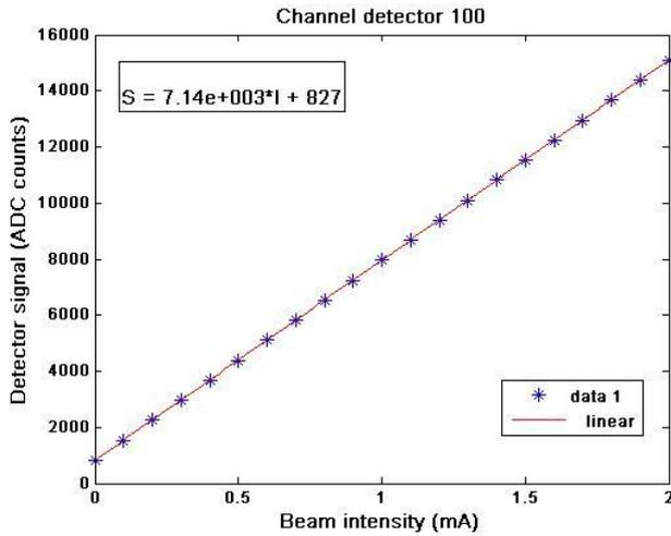
Figure 6. Dependence of detector (element number 100) response with beam intensity.
