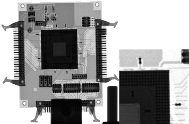
Figure 9. Digital radiography and detail of a printed circuit board with a FPGA chip.
