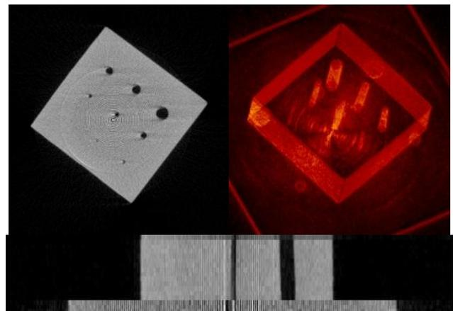
Figure 8a. (up, left) CT slice of a PMMA phantom extracted from the 3D data set (up, right) and frontal view (down).
