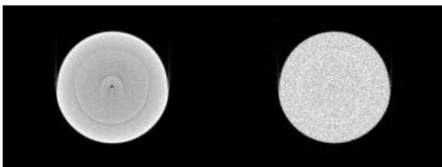
Figure 7. Beam hardening effect on a slice of a plastic cylinder (left) and filter correction (right).
