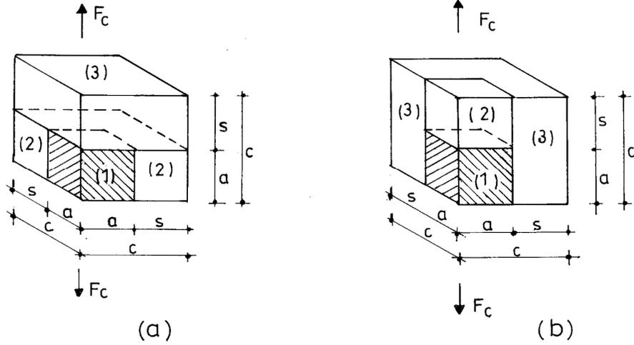
**Fig. 2** The two cube-within-cube models each consisting of three components
