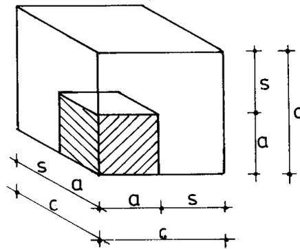
**Fig. 1** A schematic representation of the cube-within-cube model.
