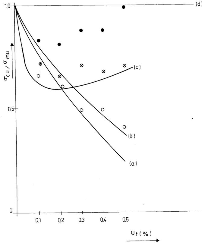
**Fig. 4** Ratio  $\frac{\sigma_{cu}}{\sigma_{mu}}$  as a function of the volume fraction filler  $u_f$ . 6,2  $\mu$ m particles
