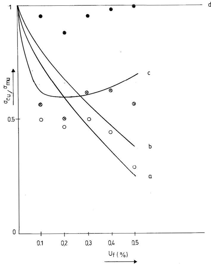
**Fig. 3** Ratio  $\sigma_{cu}/\sigma_{mu}$  (strength of the composite over strength of the matrix) as a function of the volume fraction filler  $u_f$ . 4,5  $\mu$ m particles
