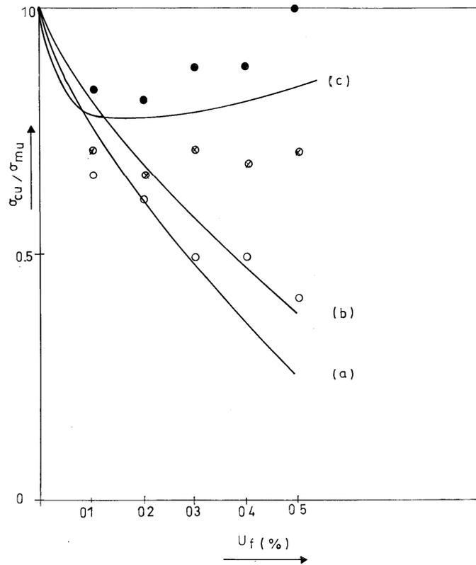
**Fig. 3.** Ratio  $\frac{\sigma_{cu}}{\sigma_{mu}}$  as a function of volume fraction of filler,  $u_f$ ,  $4,5 \mu_m$  particles
