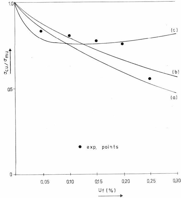
**Fig. 2.** Ratio  $\frac{\sigma_{cu}}{\sigma_{mu}}$  (strength of the composite over strength of the matrix.) versus filler volume fraction,  $u_f$ , in epoxy / iron particulate composites. (a); Nicolais and Narkis (eqs. A.4), (b); Nielsen (eqs.A.1), (c); Present model, Nielsen, (eqs. A.2 and A.3).
