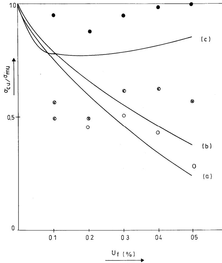
**Fig. 4.** Ratio  $\frac{\sigma_{cu}}{\sigma_{mu}}$  as a function of volume fraction of filler,  $u_f$ ,  $62 \mu_m$  particles
