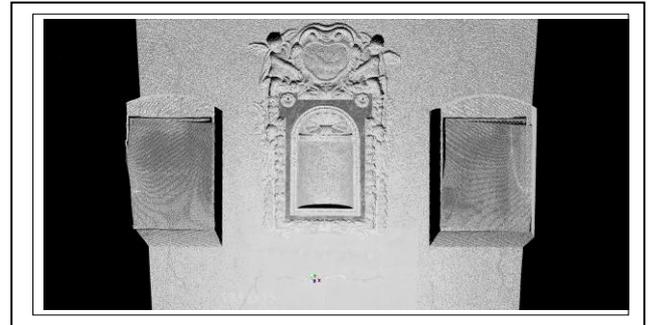
**Figure 2** – Example of 3D TLS modelling of a damaged altar of the Santa Chiara church which was subjected to restoration in the past. A test survey was done by means of Leica HDS-2500 TLS. Data were processed with the aid of Leica Cyclone Vs 5.7 software.
