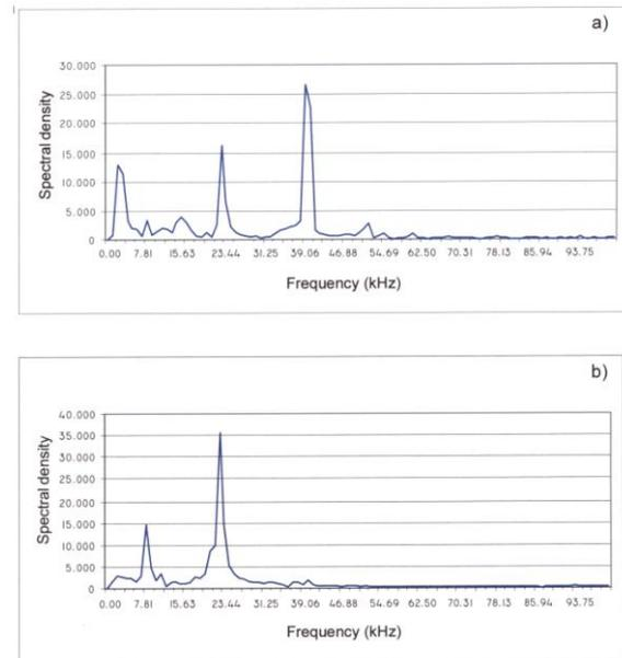
Fig.4 - FFT spectra of the ultrasonic waveforms acquired in an unaltered (a) and altered (b) sectors of the investigated masonry.
