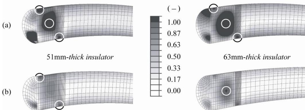
Figure 6 : Damage index for the 51mm- and 63mm-thick insulators (a) at the ultimate mechanical loading and (b) at 60 or 50%, respectively, of this load (a circle indicates highest index location)
