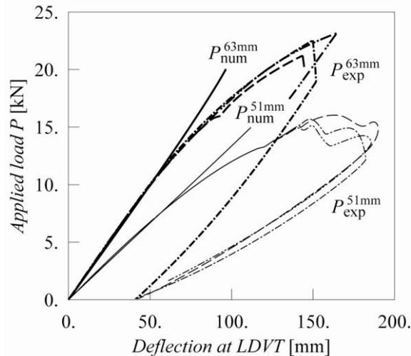
Figure 5 : Numerical and experimental load-displacement curves for the insulators investigated
