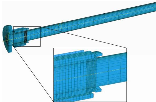
Figure 3 : Finite element model of a 63mm-thick insulator
