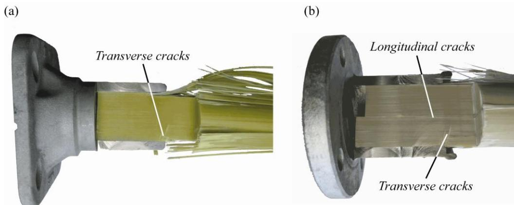
Figure 8 : Damage mechanisms for the (a) 51mm- and (b) 63mm-thick insulators
