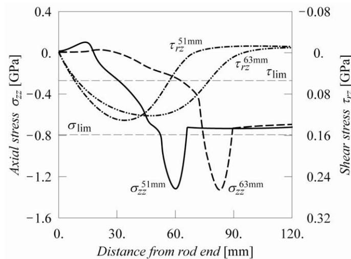
Figure 4 : Numerical stress distributions in the composite rod at the ultimate loading
