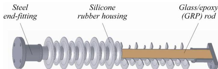
Figure 1 : Composite insulator
