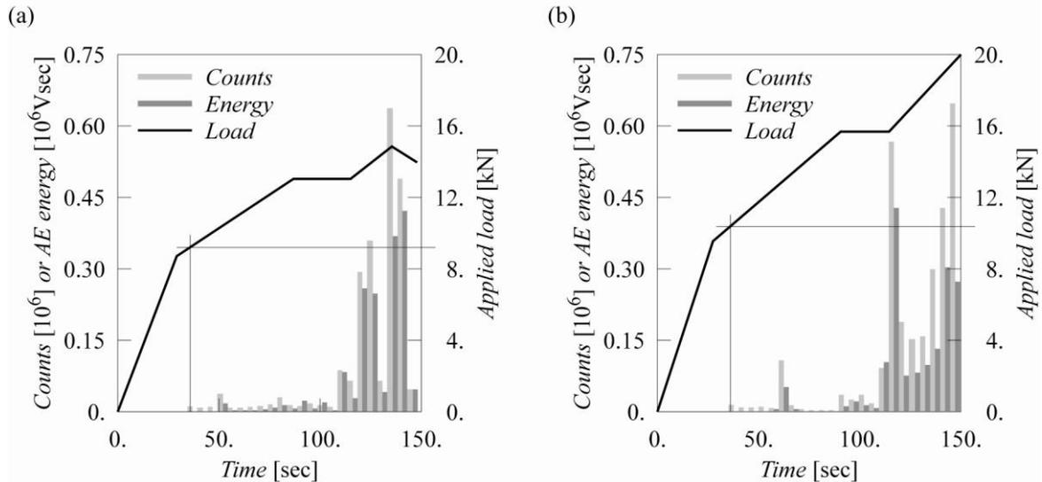
Figure 7 : Acoustic emission (AE) activity during bending of the (a) 51mm- and (b) 63mm-thick insulators
