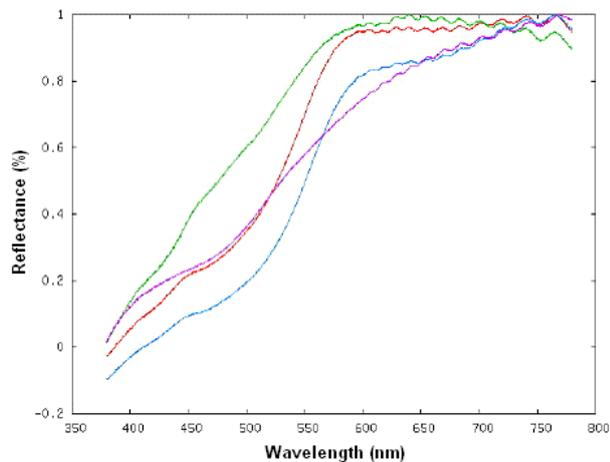
Figure 9: Spectral Reflectance of yellow stimuli in situ (mauve line), blend of lead oxide and yellow ochre JFLES (green line), yellow ochre JFLES (red line) and blend of hematite and yellow ochre JFLES (blue line).
