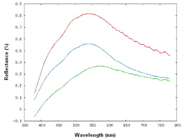
Figure 3: Spectral Reflectance of malachite on white lead substrate (red line), with an intermediate varnish layer (blue line) and without substrate (green line).
