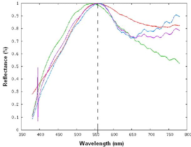
Figure 8: Spectral Reflectance for Green Stimuli in situ (red line), for malachite (green line), green earth (blue line) and a 1:1 mix of the two pigments (mauve line).
