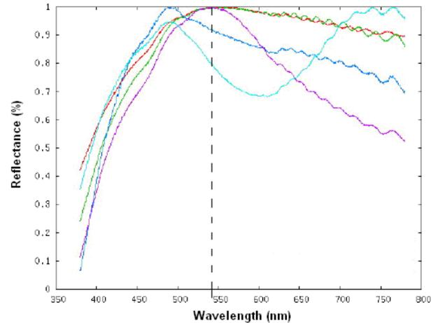
Figure 6: Spectral Reflectance of blue stimuli in situ (lines green and red), for azurite (blue line), for malachite (mauve line) and ultramarine (turquoise line).
