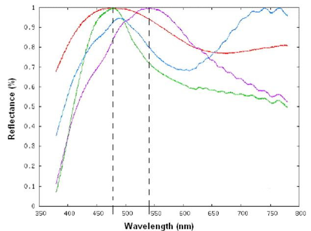
Figure 7: Spectral reflectance of blue stimuli in situ (red line), azurite (green line) and malachite (mauve line).
