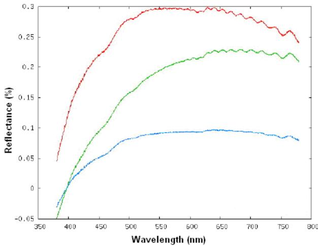
Figure 4: Spectral Reflectance of black pigment on white lead substrate (red line), with an intermediate varnish layer (blue line) and without substrate (green line).
