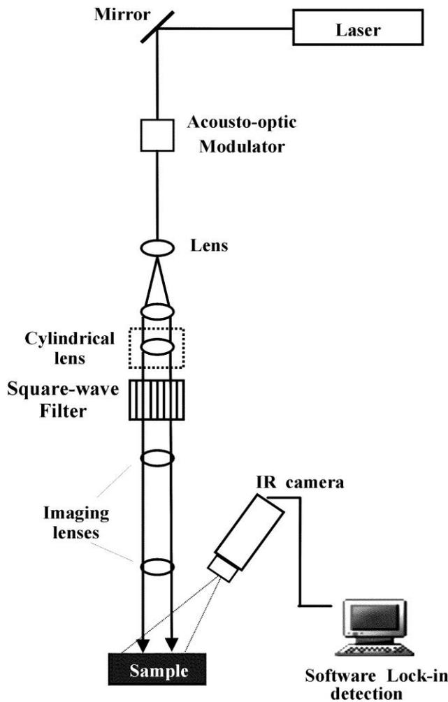
Figure 4: Experimental setup of grating IR thermography.
