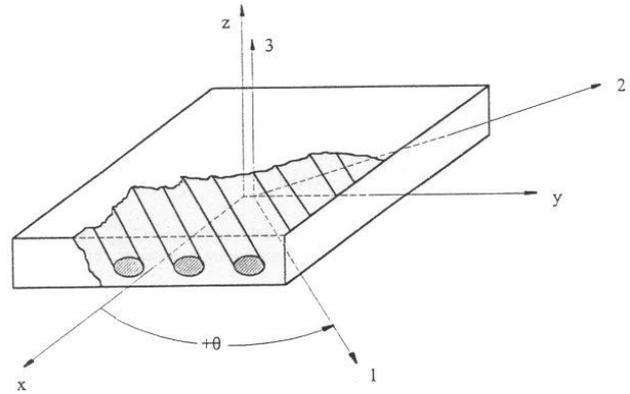
Figure 1: Rotation from the natural (global) to the principal coordinate system.
