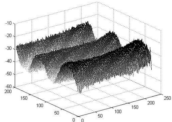
Figure 5: Phase variation at the surface of carbon/epoxy excited at 0.02Hz.
