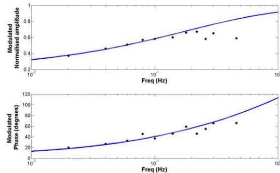
Figure 6: Manual fitting of the experimental data with the theoretical curves of the modulated temperature amplitude and phase for a carbon/epoxy laminate and a grating of 4mm.
