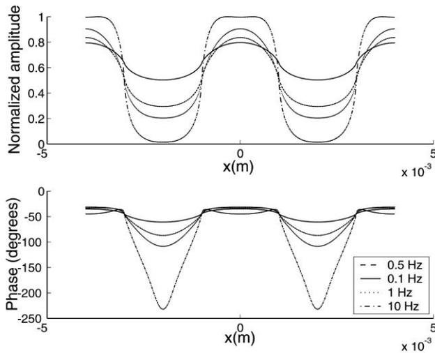
Figure 2: Normalized amplitude and phase modulation of temperature perpendicular to the grating bands ( $\lambda=4\text{mm}$ ) and the fibers as a function of frequency. The material is semi-infinite unidirectional composite with  $k_{\perp}=1\text{W/mK}$ ,  $C=800\text{J/kgC}$  and  $\rho=1550\text{kg/m}^3$  in contact with air.
