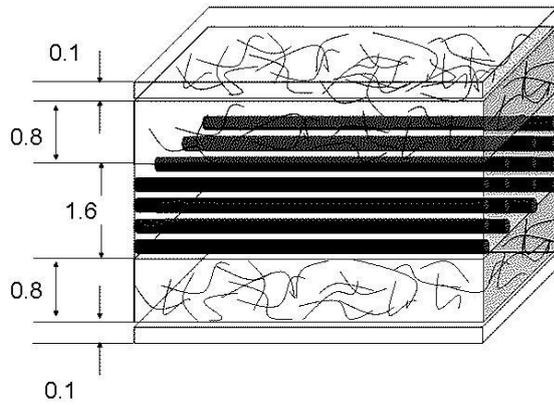
Figure 1. The stacking sequence of the tested composite material (the dimensions are given in mm).
