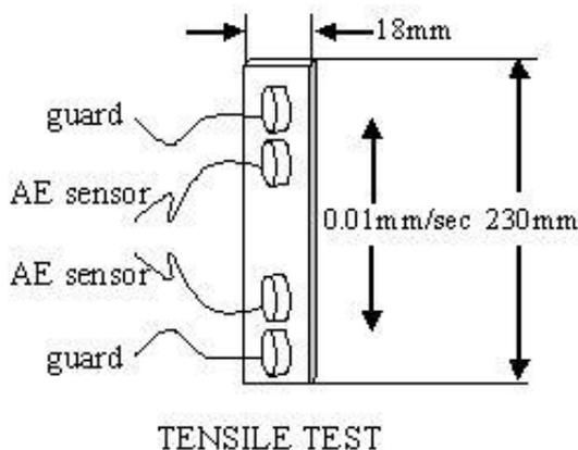
Figure 2: The experimental configuration used for tensile testing of pultruded Glass/Polyester rectangular thin specimens.
